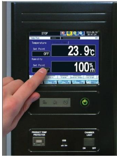
Figure 4.3 Espec Temperature Chamber Touch Screen ( Global-N Temperature Cycling Chambers )
