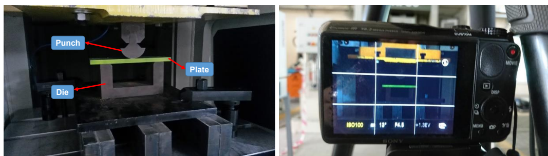
(a) (b) Figure 4.1: (a) Experimental die set (b) Set-up for image record
