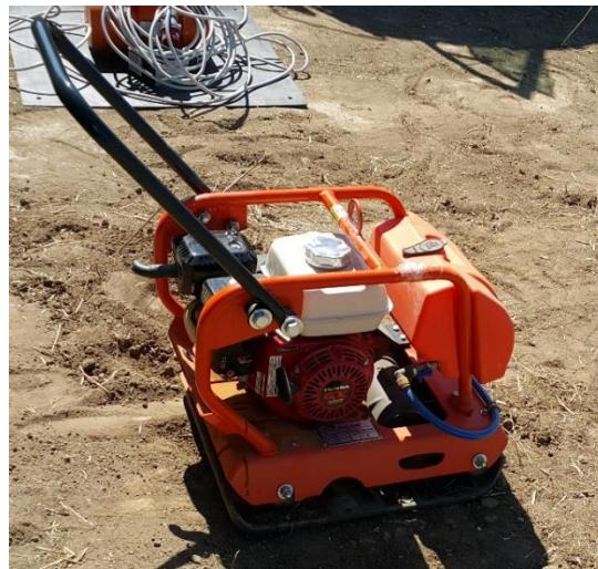
**Figure 3.8. Soil compactor vibrator**
