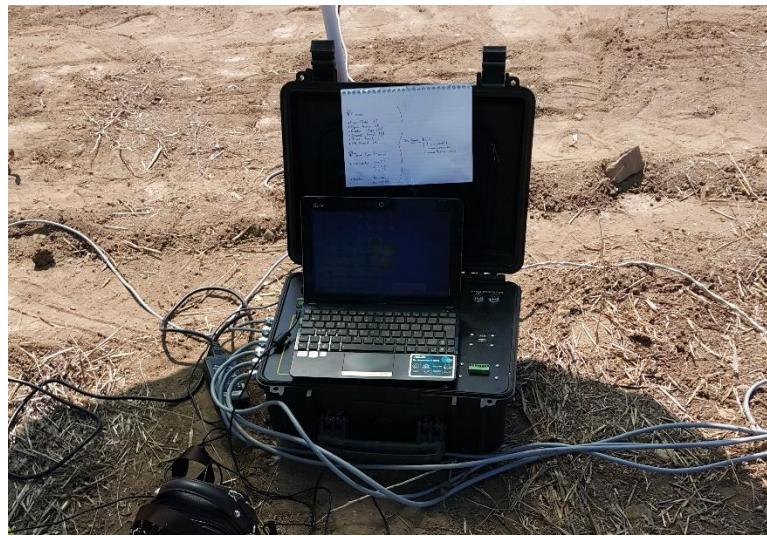
**Figure 3.16. Data acquisition logger connected to sensors**
