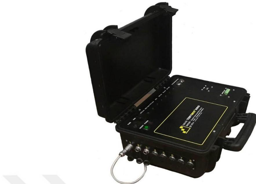
**Figure 3.11. Test Box 2010 dynamic data logger**
