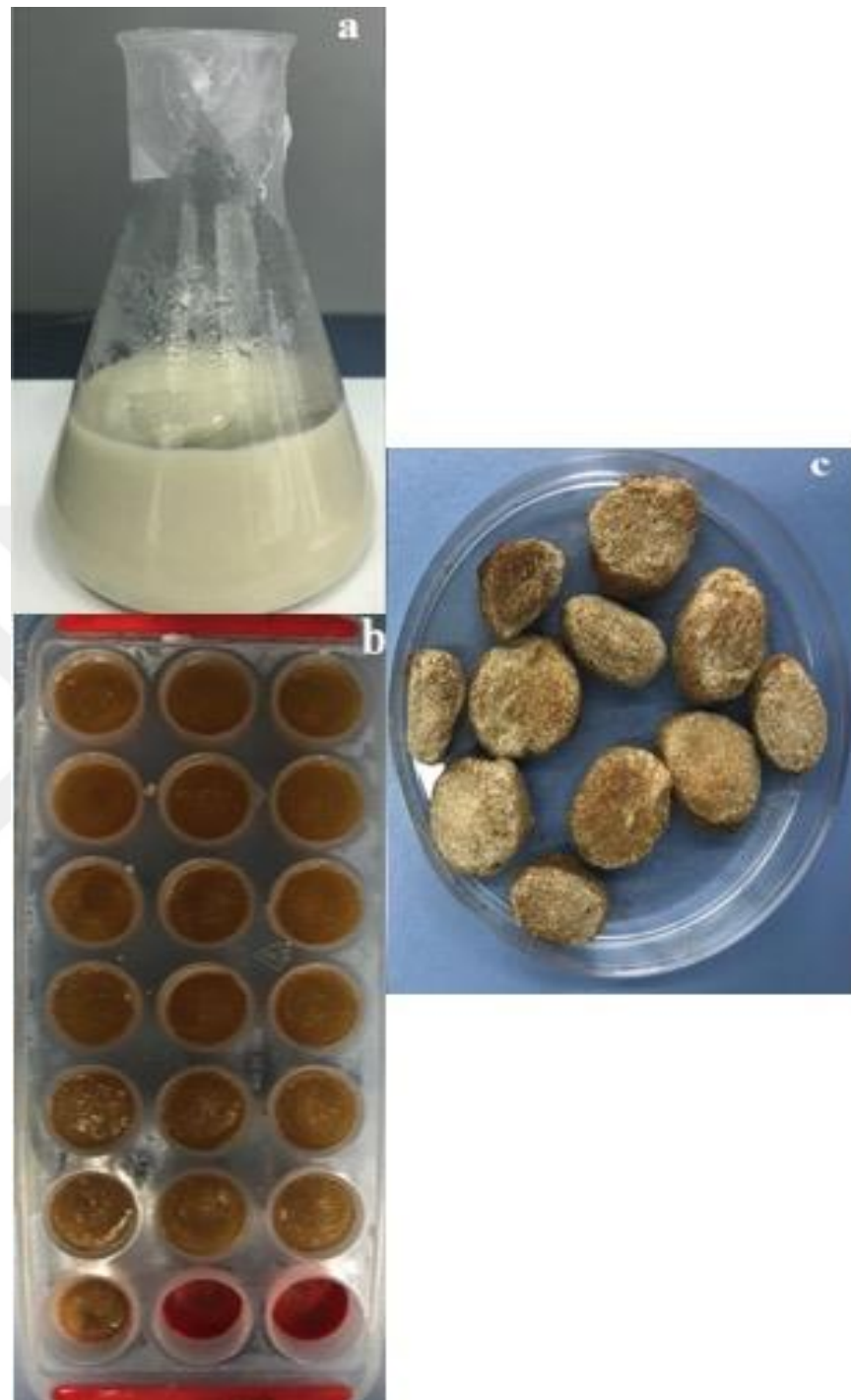
Figure 3.13. Experimental procedure; a) mixing of the components, b) molding and freezing and c) produced scaffolds after drying procedure
