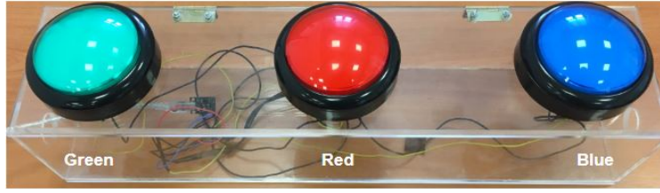
Figure 6.3: Transparent three-button box used by the participants to start the robot motion (green) and make an object guess (red and blue).
