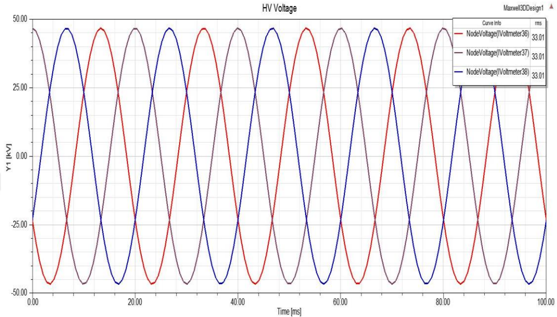
Figure 31: HV Line Voltage
