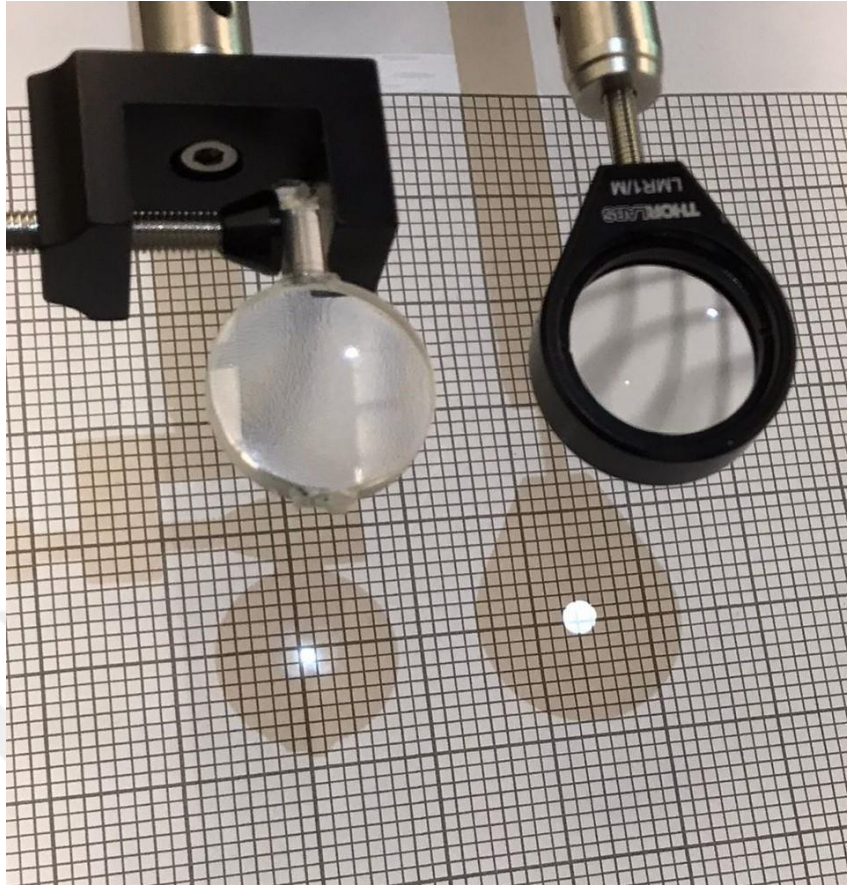
Fig. 4.2.6: PAC046 original lens and epoxy based copied lens focusing the light from crown side.
