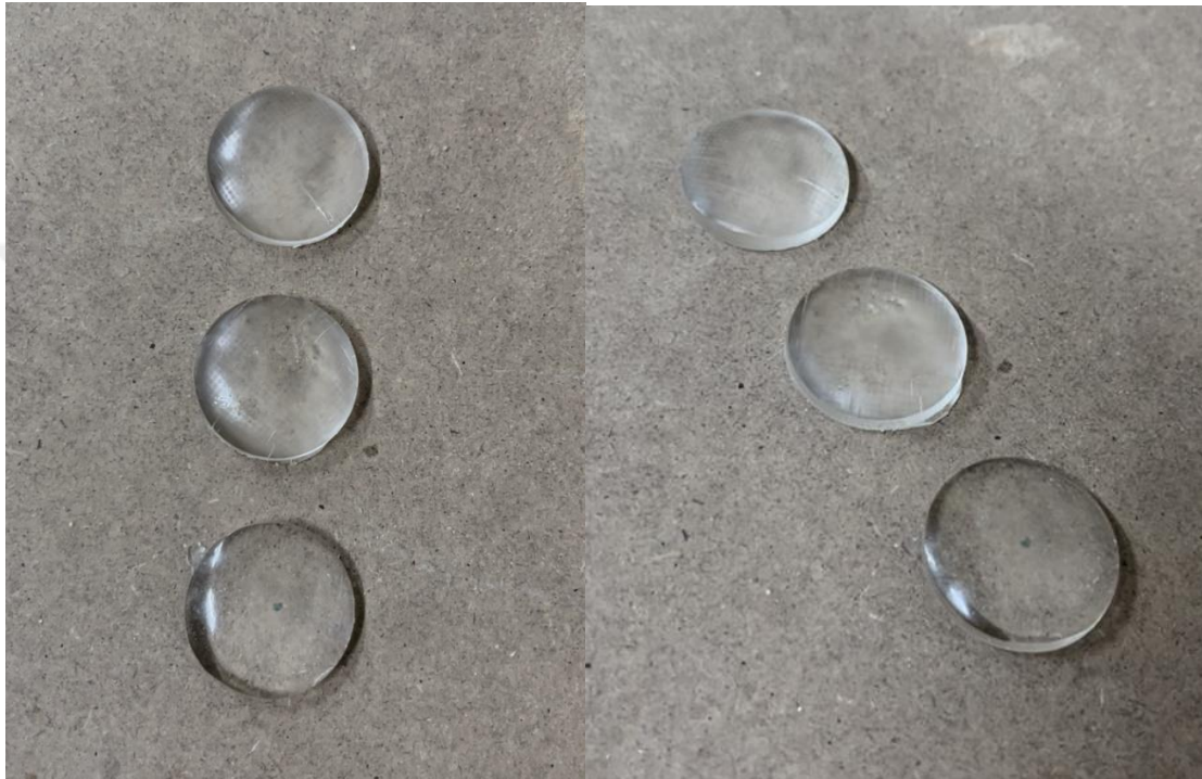
Fig. 5.1.1: First manufactured epoxy based lenses.
