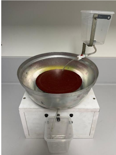
Figure 2.1.2.3: Flat lap machine Picture from behind to show water dump.
