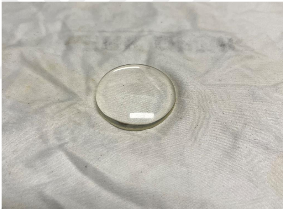
Figure 2.1.3.1. Epoxy lens that has undergone sanding and polishing processes.
