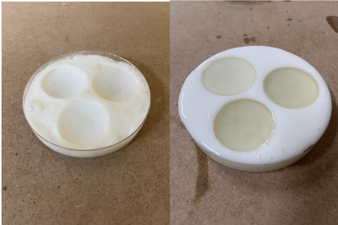
Figure 2.1.4.1. Recesses and epoxy casting of lenses molded from mold silicone.
