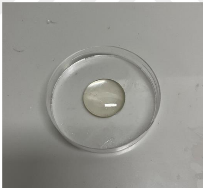
Figure 2.1.2.6: The final state of the lens that comes out of the 3D printer, which has been sanded and polished.
