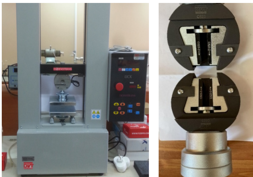
Figure 2.6: Tension-compression test device
