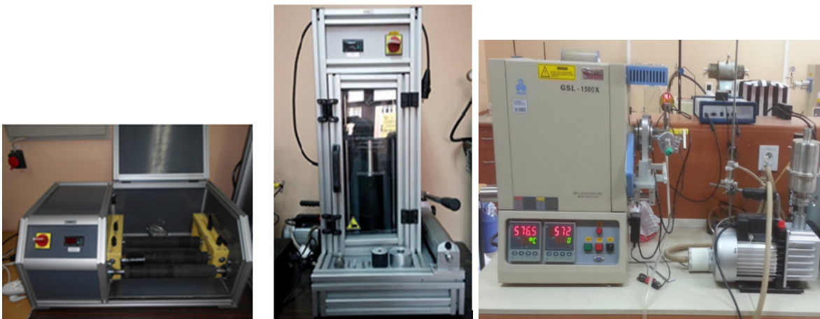
Figure 2.4: a) Ball mill and hydraulic press, b) sintering furnace
