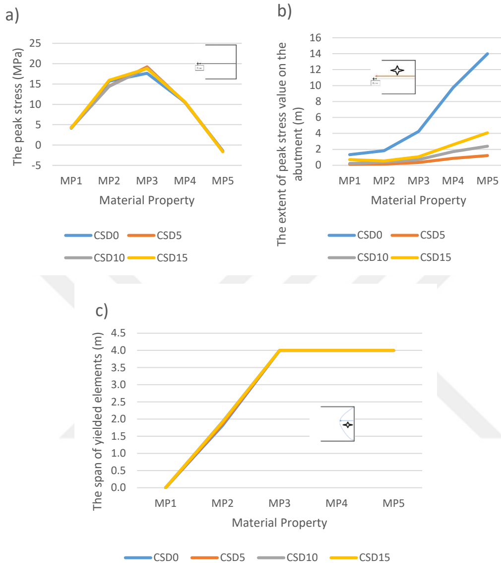
Figure G. 4 a) Peak Stress, b) The Extent of Peak Stress Value on The Abutment, c) The Span of the Yielded Elements vs. Material Properties for Left Abutment
