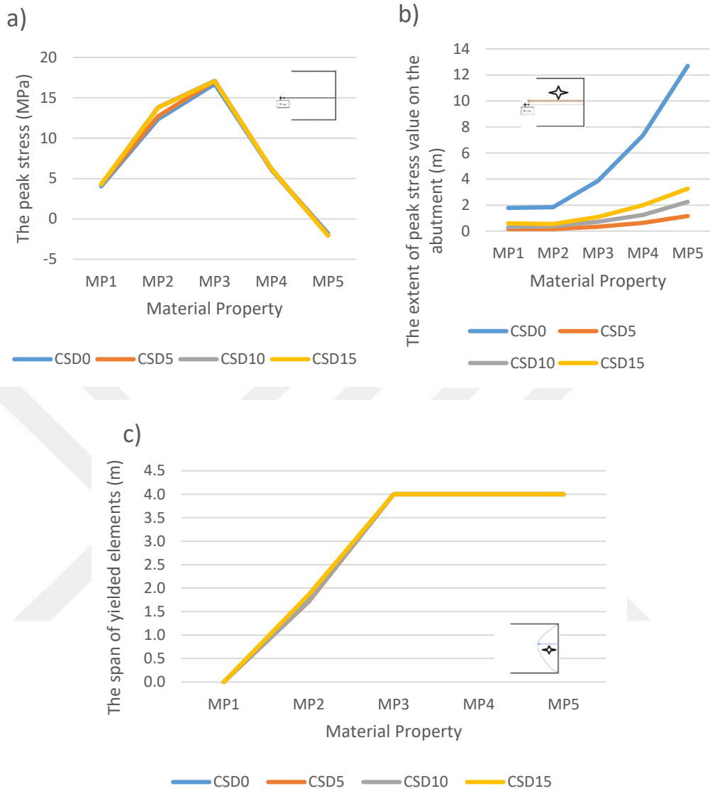
Figure H. 4 a) Peak Stress, b) The Extent of Peak Stress Value on The Abutment, c) The Span of the Yielded Elements vs. Material Properties for Left Abutment
