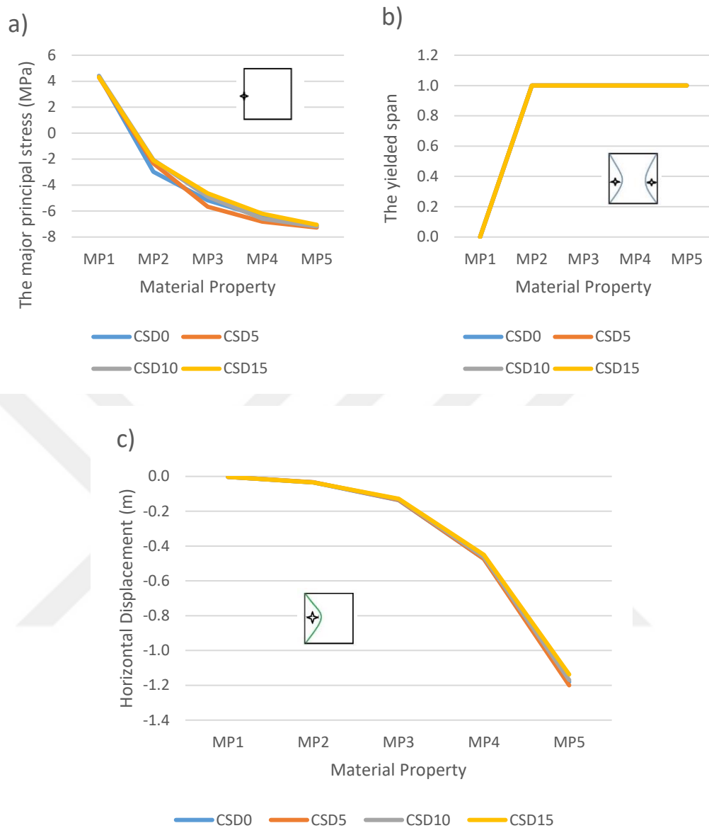
Figure G. 3 a) Major Principal Stress, b) Yielded Span, c) Horizontal Displacement vs. Material Properties for Right Pillar
