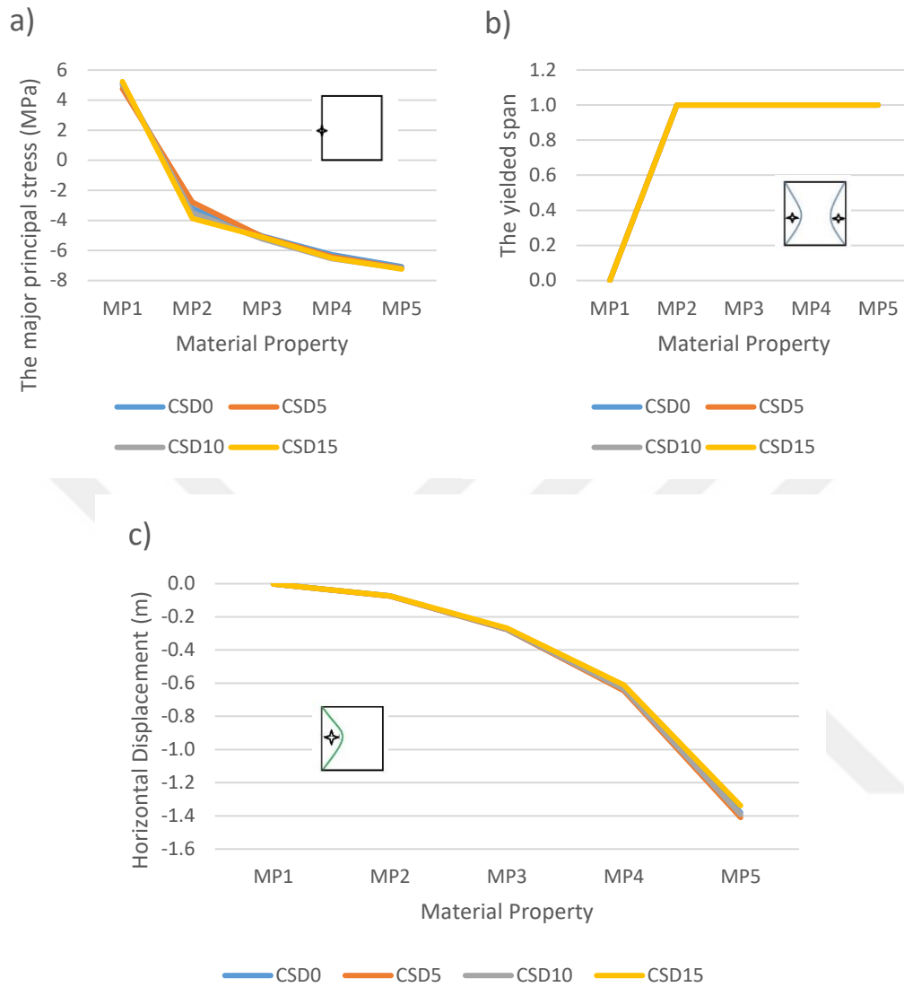
Figure G. 2 a) Major Principal Stress, b) Yielded Span, c) Horizontal Displacement vs. Material Properties for Center Pillar
