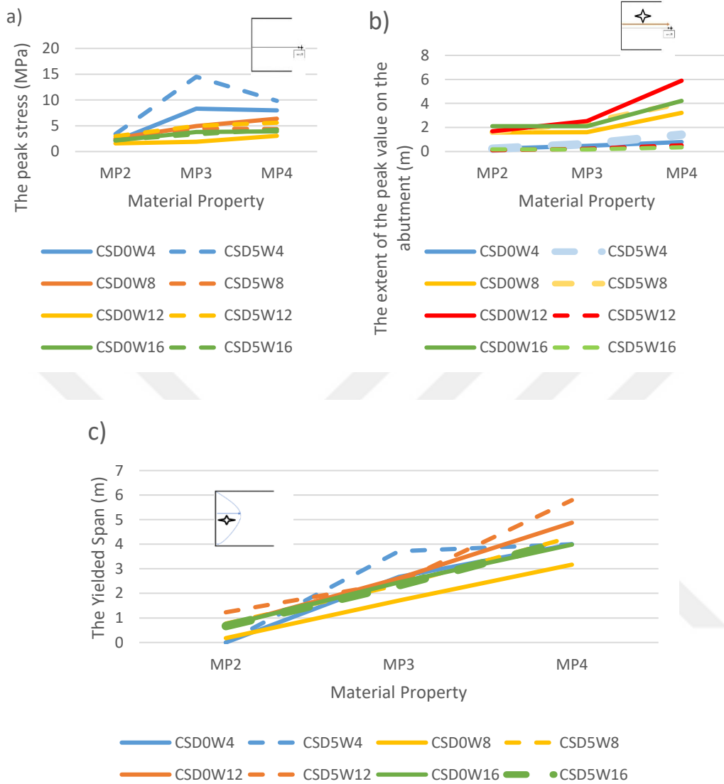
Figure E. 5 a) Peak Stress, b) The Extent of Peak Stress Value on The Abutment, c) The Span of the Yielded Elements vs. Material Properties for Right Abutment
