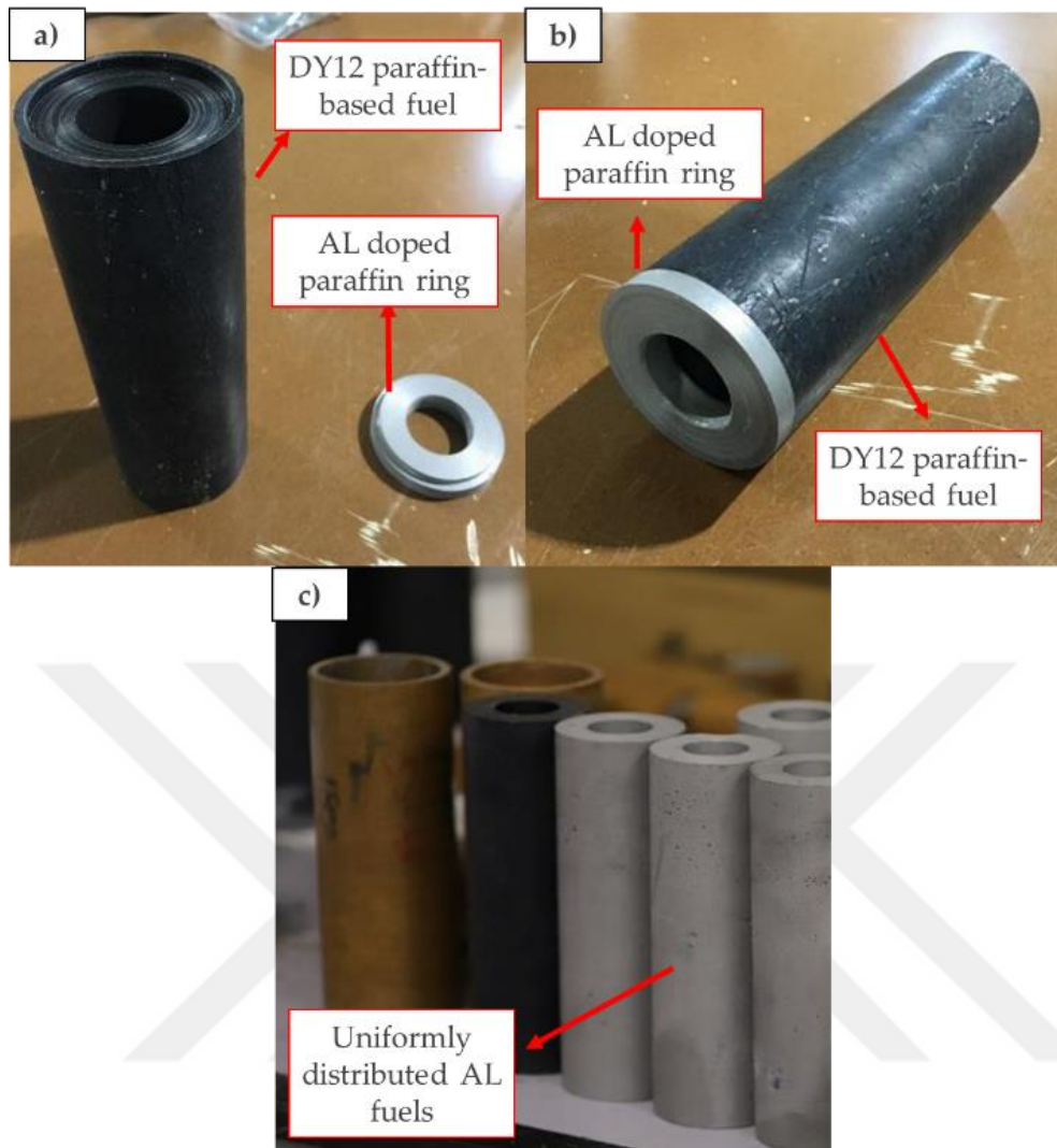
Figure 5.4 : Hybrid rocket fuels used in the tests: a) Aluminum added fuel ring and paraffin-based fuel, b) Al ring attached to the front of the paraffin-based fuel, c) Uniformly distributed Al fuels.
