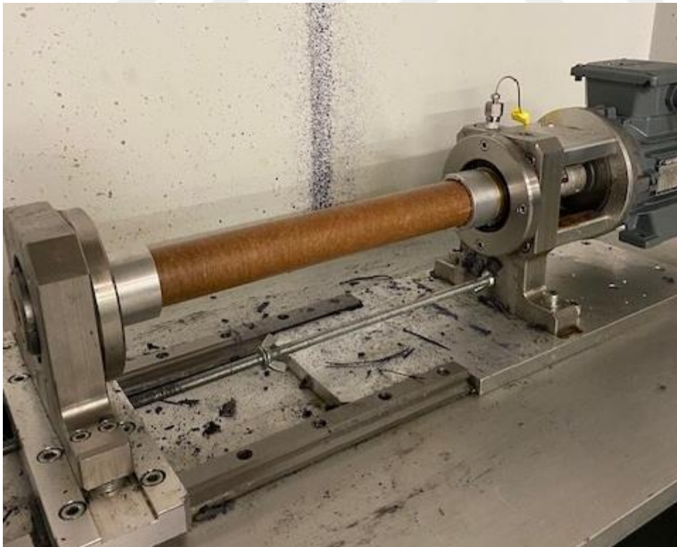
Figure 3.8 : Spin casting machine and phenolic fuel case.
