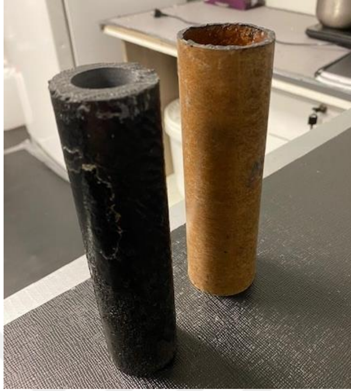
Figure 3.9 : Paraffin-based fuel and phenolic casing.
