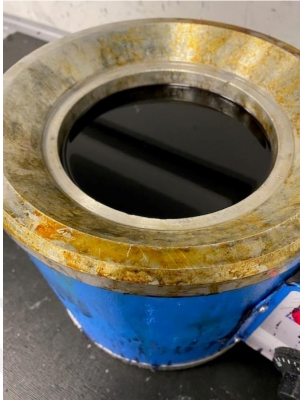
Figure 3.7 : Liquid form of the paraffin-based fuel.
