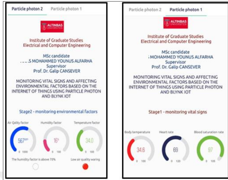
Figure 3.19: Screen Shot of Blynk Interface of the System.
