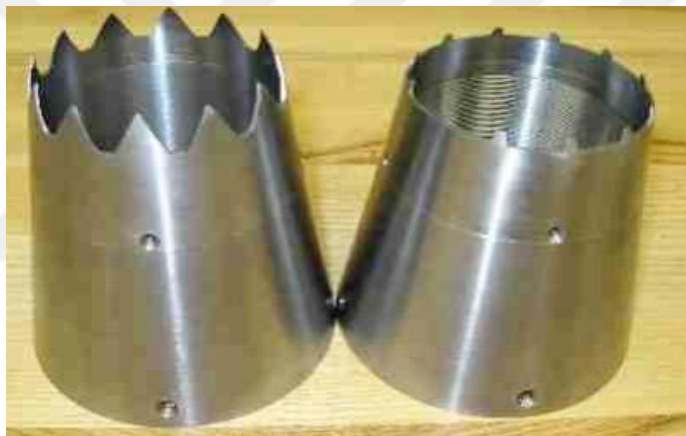
Figure 1-8 The left one is chevron nozzle and the right one is tabbed nozzle [18]
