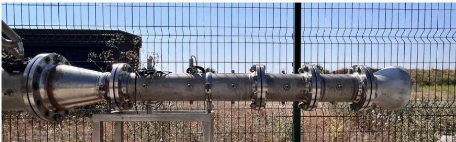
Figure 4-12 Ejector-Diffuser section in setup
