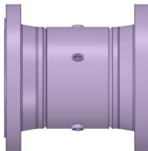
Figure 4-9 CAD model of the spool component
