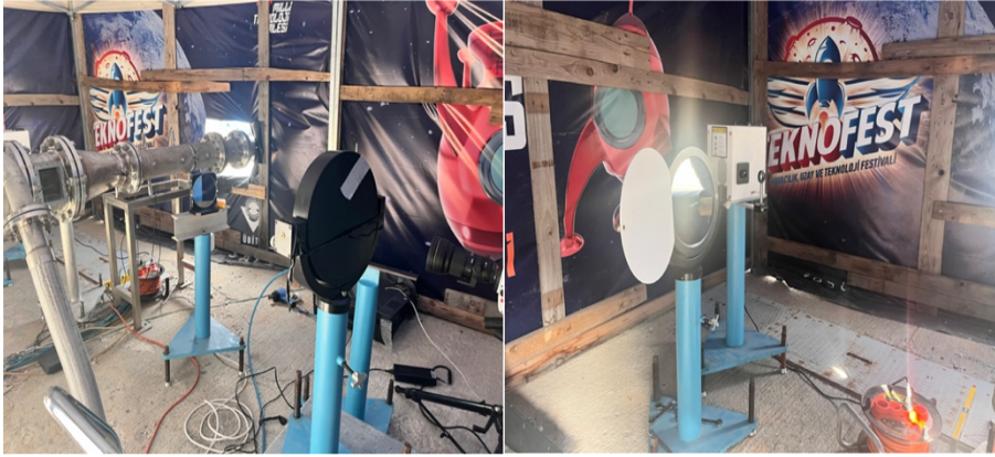
Figure 4-27 Mirror positions of Schlieren setup
