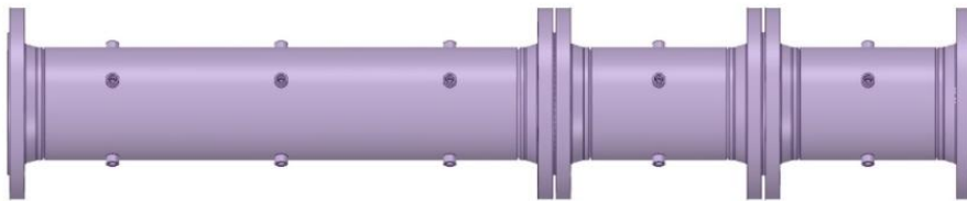
Figure 4-11 CAD model of ejector-diffuser
