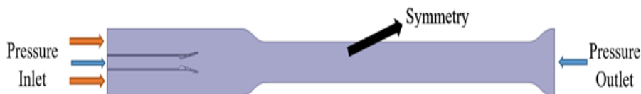
Figure 3-3 Boundary definitions of ejector system
