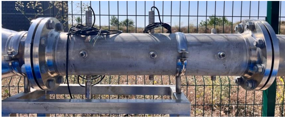
Figure 4-13 Ejector-Diffuser section's body component in setup
