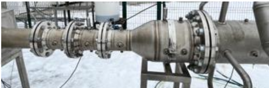
Figure 4-6 Test chamber diffuser in setup
