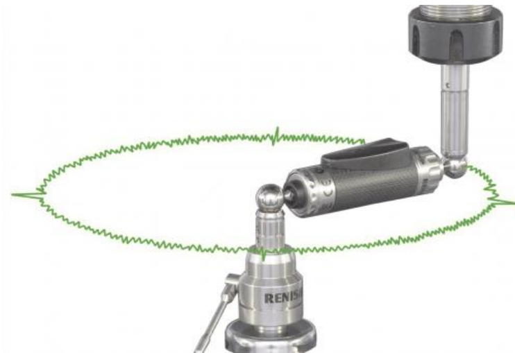
Figure 6: Ballbar test calibration
