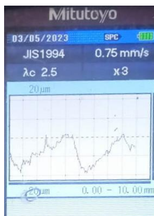
Figure 11: Surface roughness measuring, Mitutoyo SJ 210
