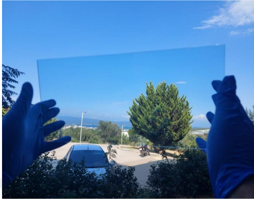
Figure 4.2. ZTO/Ag/ZTO coated on 2 mm thick glass
