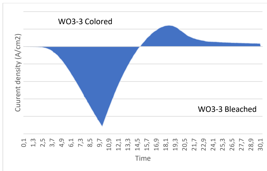
Figure 4.19. Development of current density based on CV measurement of 30 second cycle of WO 3 -3 thin film at 100 mV/s
