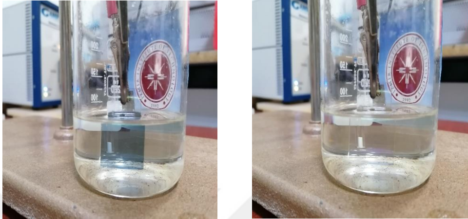
Figure 4.8. Coloration status of glass/ITO/ \text{WO}_3 deposited thin film in 1 M \text{LiClO}_4 -PC electrolyte
