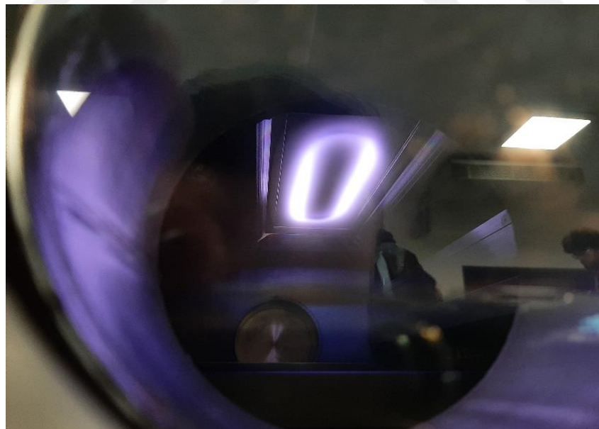
Figure 3.2. Plasma of the magnetron sputtering system
