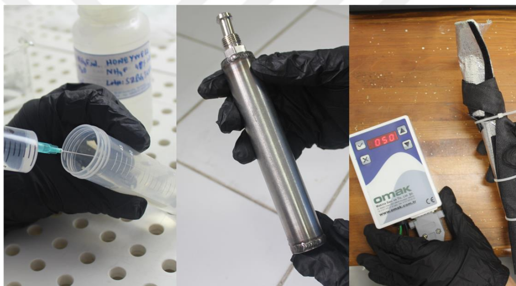
Figure 2.4 The \text{NH}_4\text{F}/\text{DI} solution adjustments for each experiment and the heater system for the canisters
