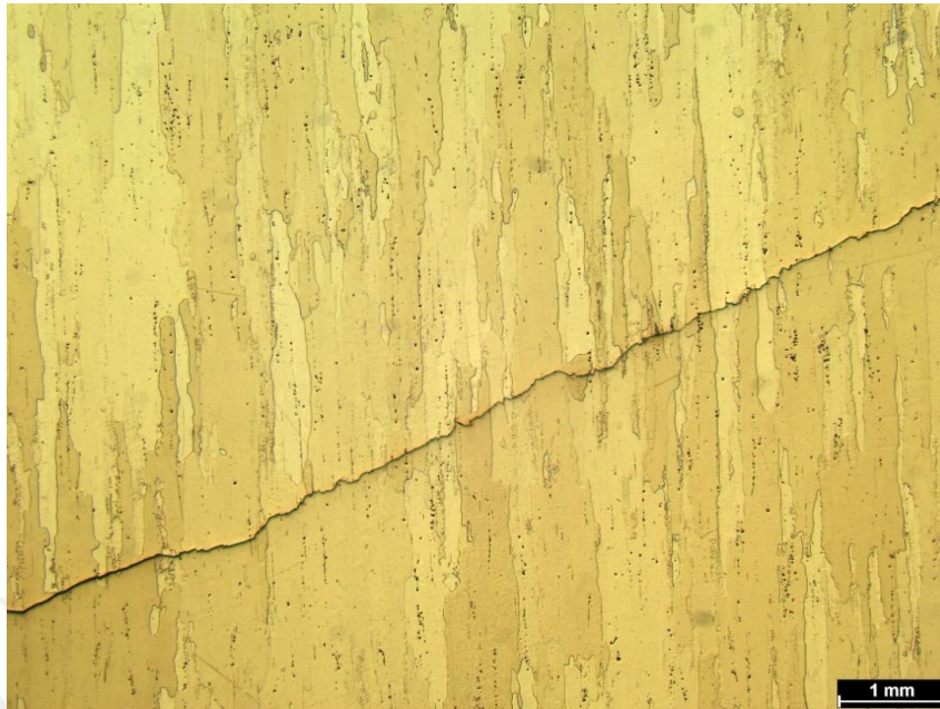
Figure 3.50. Optical microscope image of the deviated crack in P20_L-T sample.
