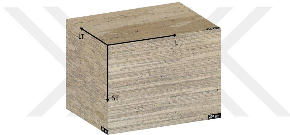
Figure 3.1. 3D microstructure of the sample extracted from the 20 mm thick plate.
