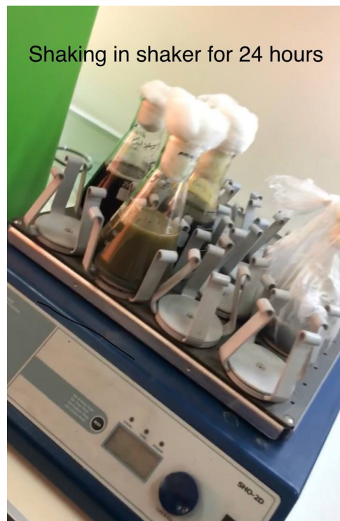
Picture 3.4. Overnight incubation in a shaker
