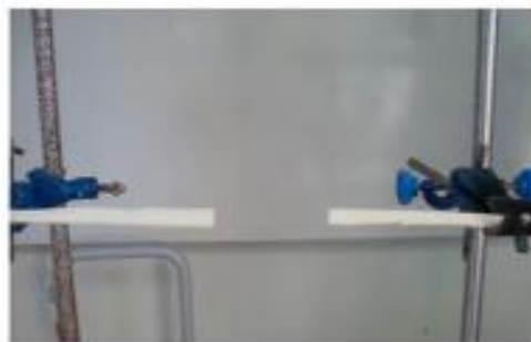
Figure 3.20 : UL-94 horizontal burning test.
