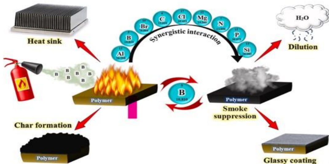
Figure 2.12 : Boron compounds fire reaction mechanism [50].
