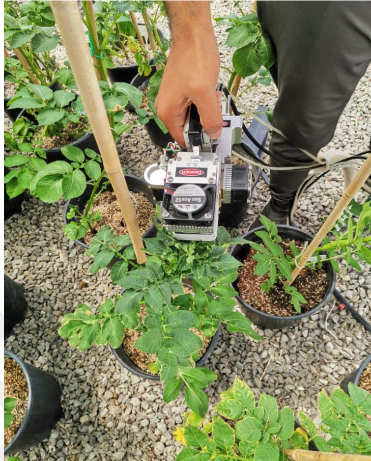
Figure 3.2. Determination of physiological traits of potatoes by using a portable photosynthesis system
