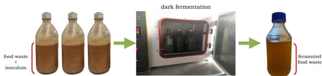
Figure 3.2 : Setup of dark fermentation process.
