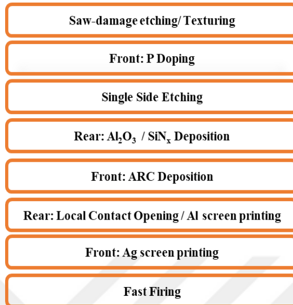
Figure 2.2 PERC Fabrication steps.
