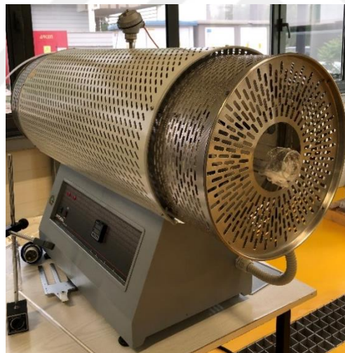
Figure 3.10 Annealing furnace with N 2 gas atmosphere.
