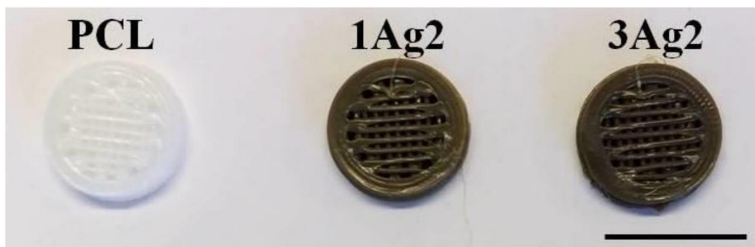
Figure 2.15 : Photograph of the PCL and PCL/AgNp 3D-printed scaffolds [74].
