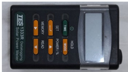
Figure 3.36. Solar power meter (TES)
