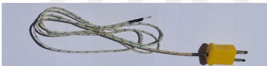
Figure 3.38. Thermocouple of type K
