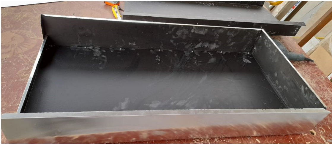
Figure 3.27. Manufacturing dual-flow SAH structure
