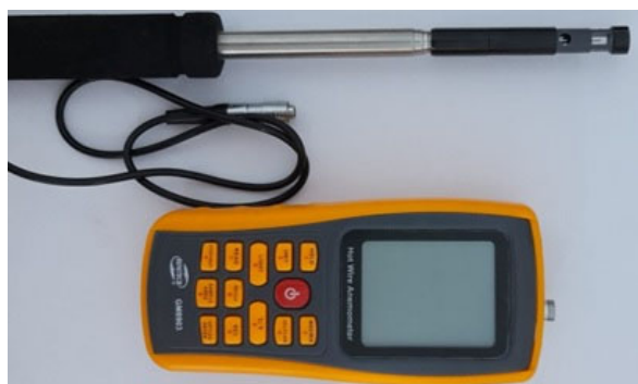
Figure 3.37. Hot Wire Anemometer GM8903
