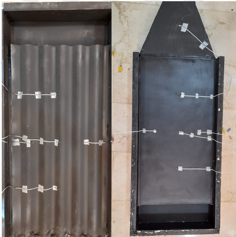
Figure 3.42. Arrangement the fixing of thermocouples
