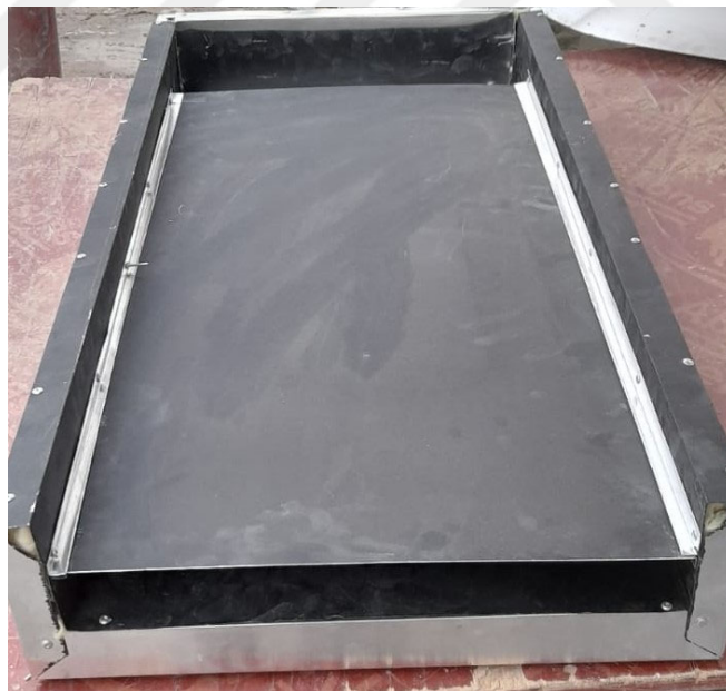
Figure 3.28. Dual-flow SAH structure
