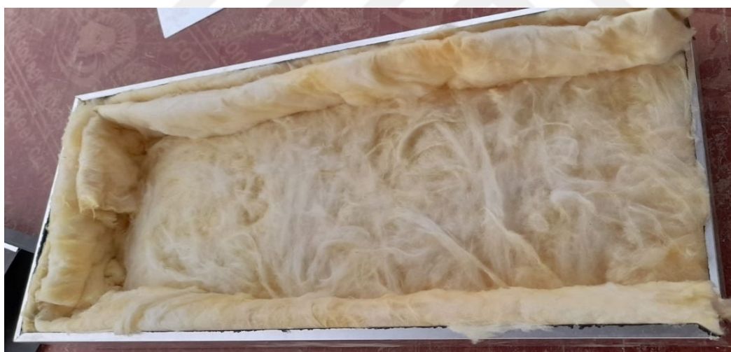
Figure 3.33. Insulation of Collector
