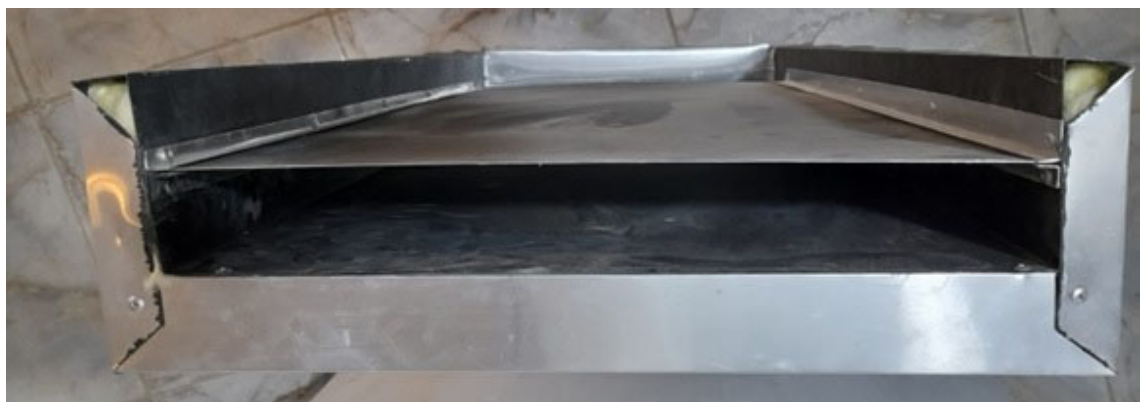
Figure 3.30. The absorber plate at 10 cm away from the SAH base
