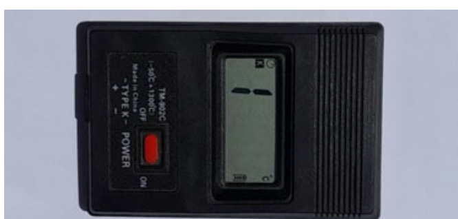
Figure 3.39. Temperature Meter TM-902C (-50C-1300 °C)
