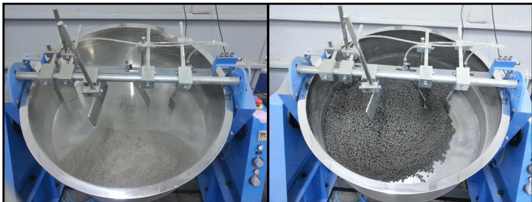
Figure 3.1. General view of the pelletizing disc and the production of fly ash aggregate.
