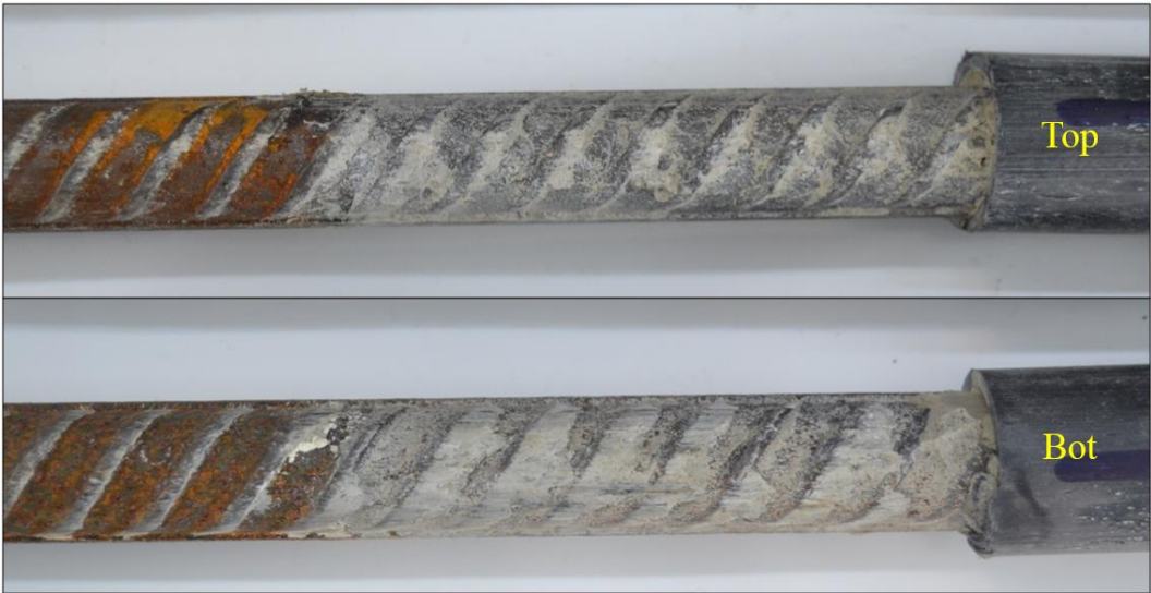
Figure 4.35. Mortar adhered on bars in a column specimen of TFAAC.
