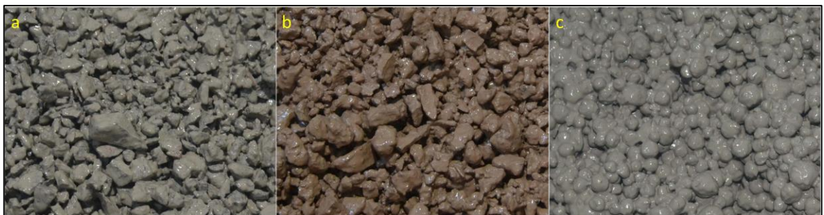
Figure 3.6. GGBFS slurry coated recycled aggregates: (a) TRCA, (b) TRBA, (c) TFAA.
