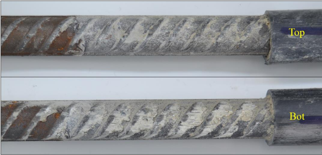
Figure 4.37. Mortar adhered on bars in a column specimen of TRCAC.
