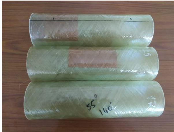
Figure 5.15 55-degree filament wound at 140°C curing temperature, and delamination
