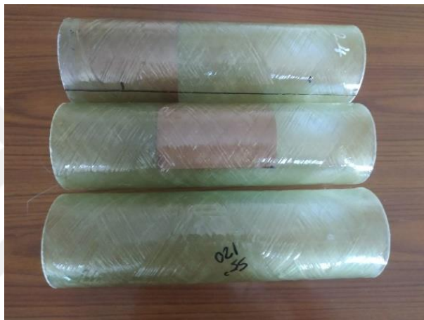
Figure 5.16 55-degree filament wound at 120°C curing temperature, and delamination
