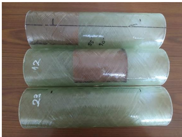
Figure 5.17 55-degree filament wound at 90°C curing temperature, and delamination
