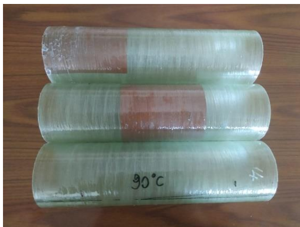
Figure 5.11 85-degree filament wound at 90°C curing temperature, and delamination
