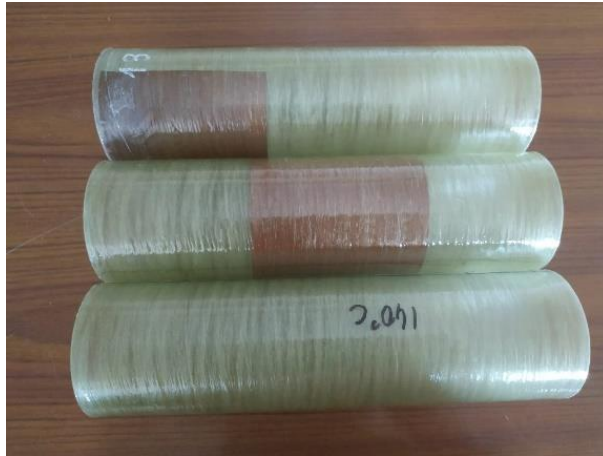
Figure 5.9 85-degree filament wound at 140°C curing temperature, and delamination
