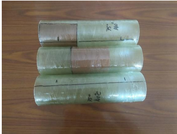
Figure 5.12 75-degree filament wound at 140°C curing temperature, and delamination
