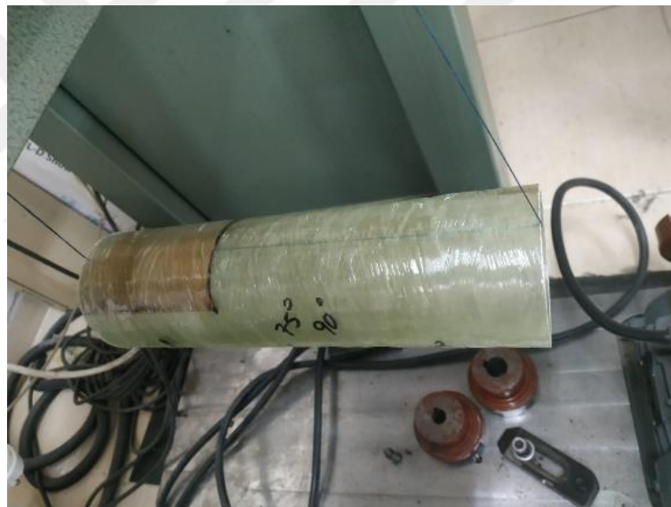
Figure 5.20 Delaminated sample testing
