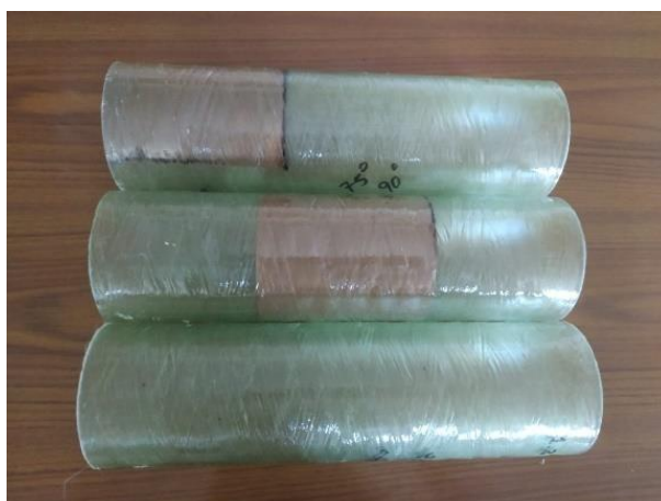
Figure 5.14 75-degree filament wound at 90°C curing temperature, and delamination
