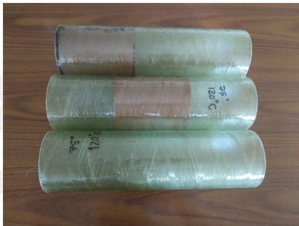
Figure 5.13 75-degree filament wound at 120°C curing temperature, and delamination
