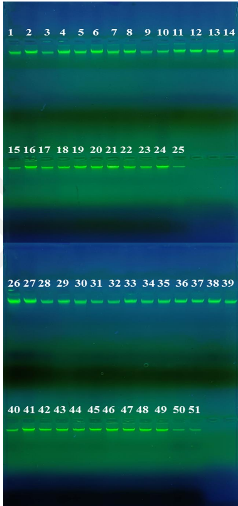
Figure 4.2 Gel electrophoresis of genomic DNA extraction from Bacteria, 1% agarose gel at 5 vol /cm for 30 min
