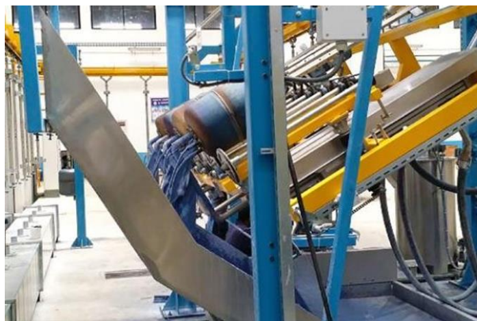
Figure 3.6 Flow Coating Method
