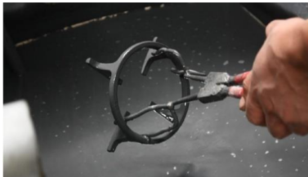
Figure 3.4 Dipping Method in the Wet Process
