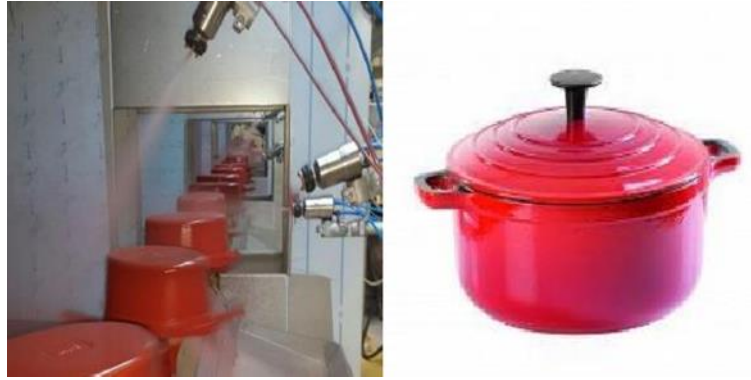
Figure 3.3 Wet Spraying Method
