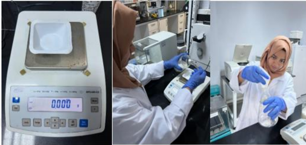
Fig.2.5. Preparation Of Mediums (Taring (Left);Measuring On Weighing Scale (Middle) And Pouring Into The Flask (Right)).
