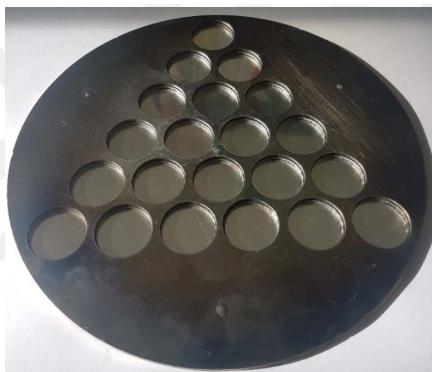
Figure 4.7 21 Ni substrates lined up on the substrate tray
