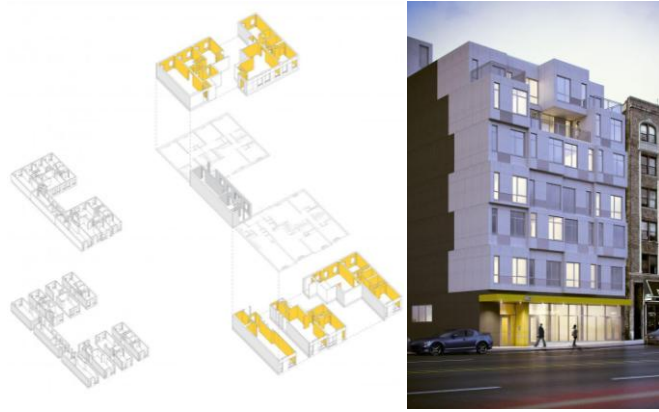
Figure 4.44: Module Combination and Image of The Stack (GLUCK+, n.d.)
