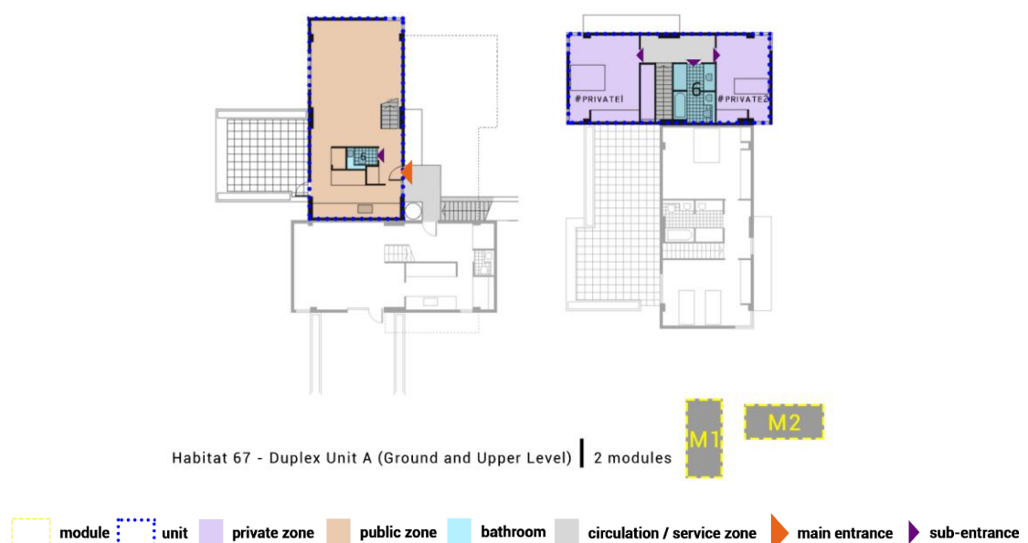
Figure 4.52: Plan Diagram of a Unit Type in Habitat 67 27
