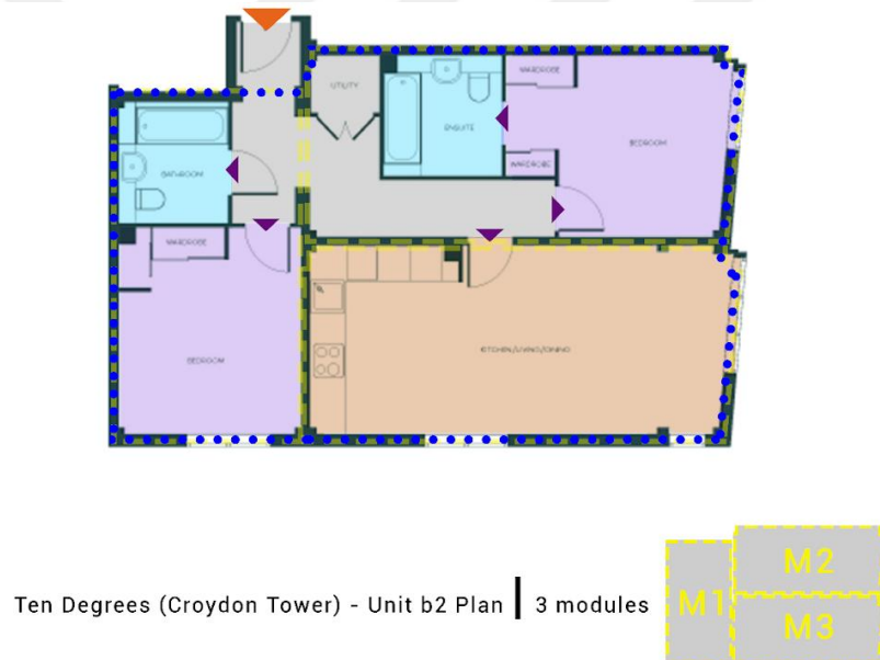
Figure 4.18: Diagram of Plan of Unit b2, Croydon Tower 14
