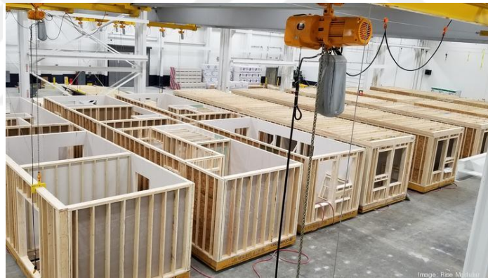
Figure 2.5: 3D Timber Modules in Production Line 4
