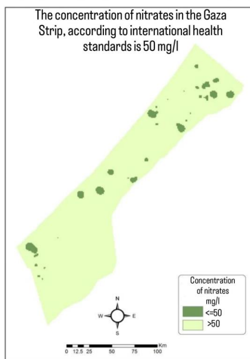
Figure 4.18 The concentration of nitrates according to the standards of the World Health Organization (50 mg/L)
