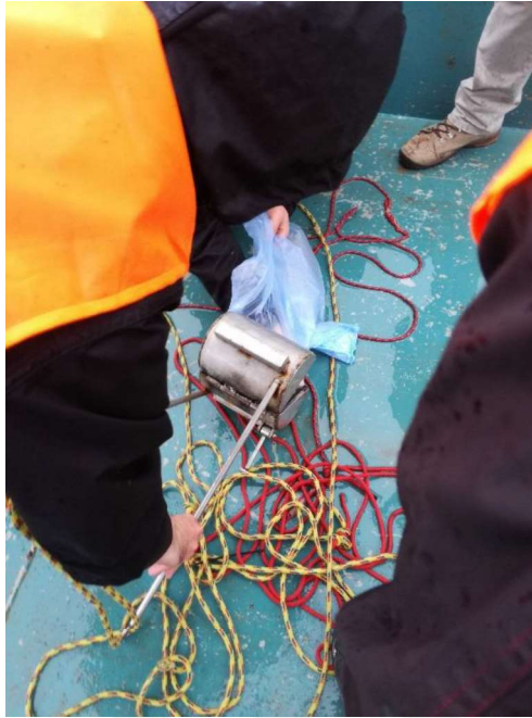
Figure 3.11 Bottom sediment sampling during the field study
