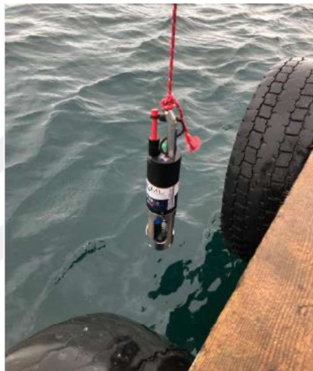
Figure 3.10 Temperature, salinity and turbidity data acquired with CTD sensor
