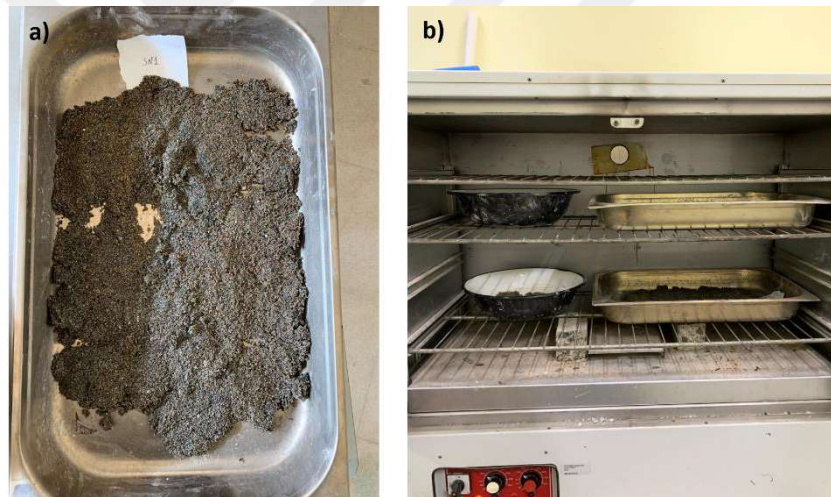
Figure 4.1 a) Bottom sediment sample, b) oven drying the samples
