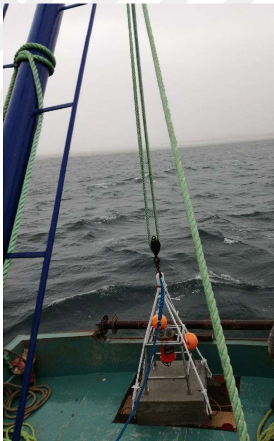
Figure 3.12 ADCP installation using a crane system during fieldwork (February 2019)
