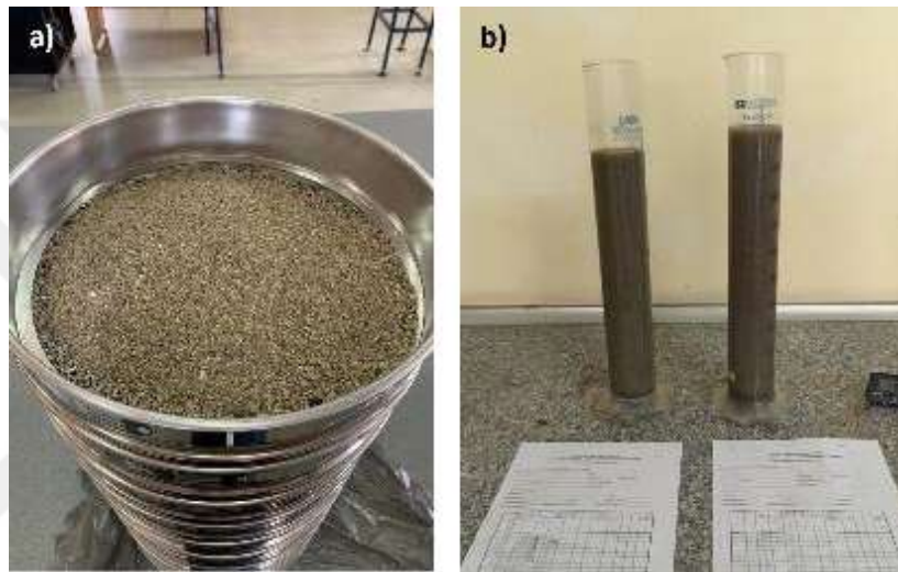
Figure 4.2 a) Sieve analysis, b) Hydrometer test
