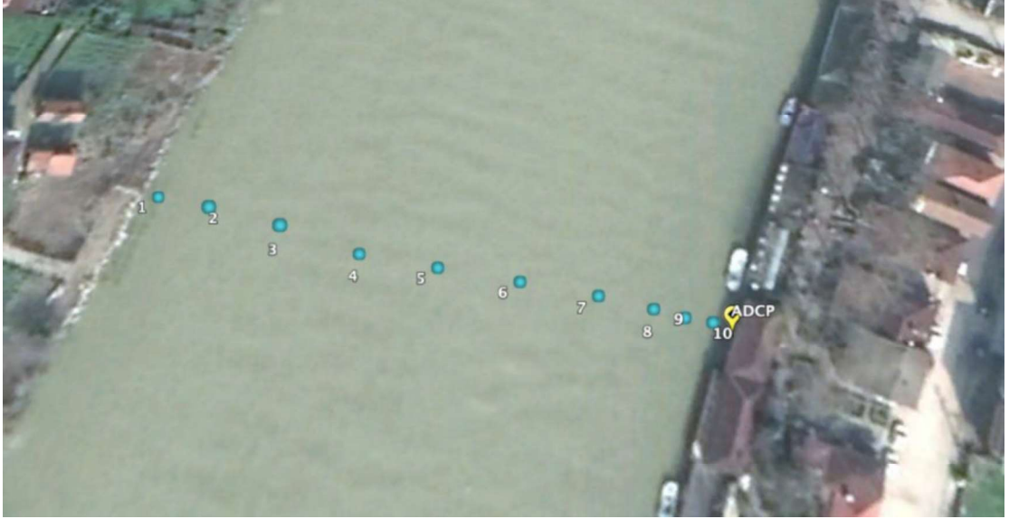
Figure 3.8 Location of measurement station for river cross-section approximately 400m distance behind the river mouth
