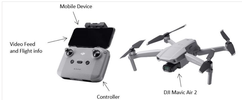
Figure 2. System overview of the DJI Mavic Air 2. ("Mavic air 2," n.d.)
