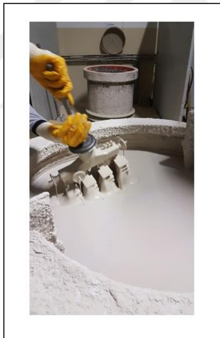
Figure 3.17 Dipping mold C into the intermediate slurry.
