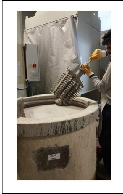
Figure 3. 11 Dipping mold A into the primary slurry.
