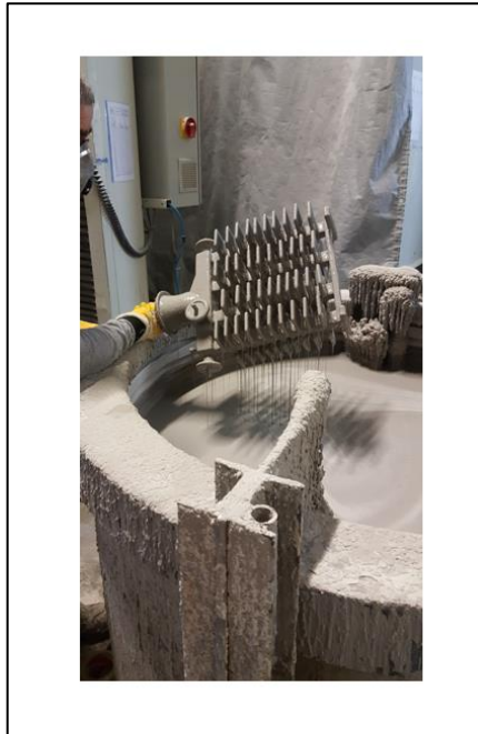
Figure 3.16 Dipping mold C into the primary slurry.
