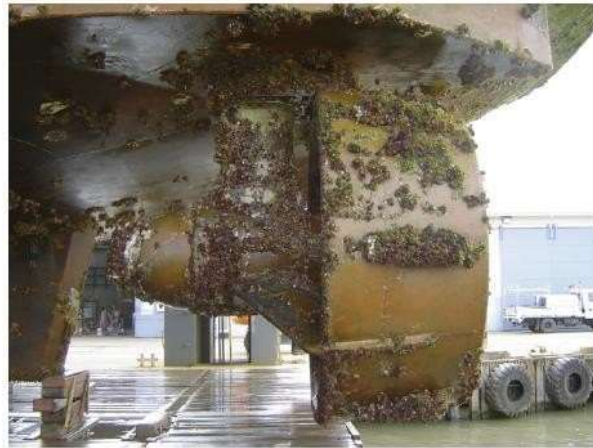
311 Figure 1: Attachment of micro-organisms, including larvae of invertebrates such as ascidians, 312 serpulids and barnacles through vessel hull fouling (Dafforn et al. 2011).
