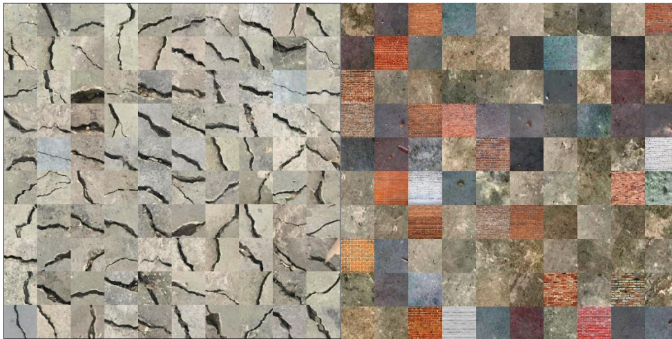
Figure 4.12 Sample of images used in training of the CNN (images with cracks at left, images without cracks at right)
