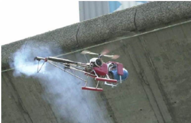
Figure 2.6 Mono camera integrated helicopter developed for bridge inspection (Metni & Hamel, 2007)
