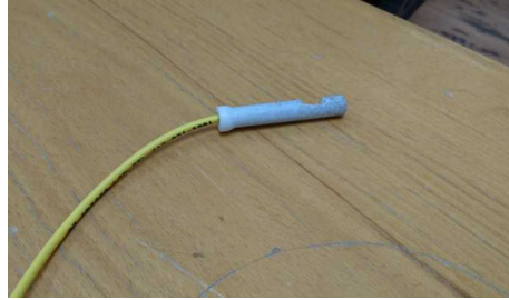
Figure 4.19: Holder used to insert the probe inside the hole drilled in engine block
