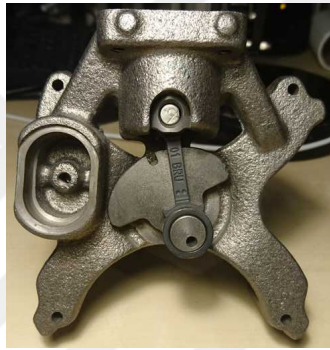
Figure 6.1: Piston and cylinder assembly of a refrigerator compressor
