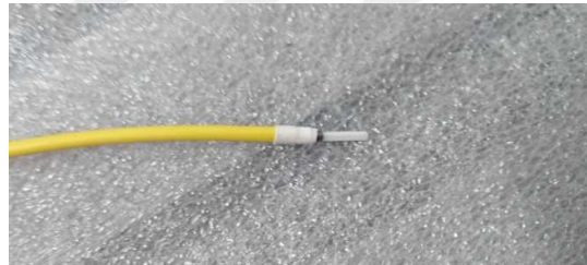
Figure 4.13: Fiber optic cable end, with polished ferrule
