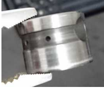
Figure 6.7: Surface of piston wet-sanded with wet-and-dry sandpaper
