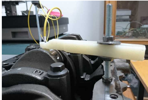
Figure 4.17: Probe holder used for the encoder probe
