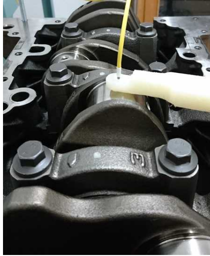
Figure 6.28: Crankpin at its closest location to the encoder probe
