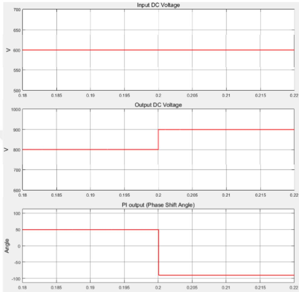
Figure 4.7. The system response to increasing output DC voltage
