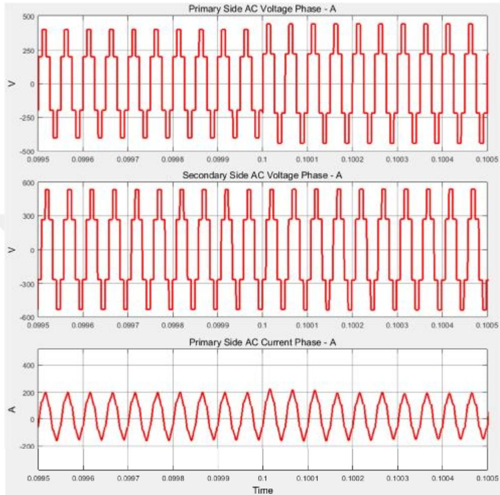
Figure 4.10. The waveforms of increasing input DC voltage
