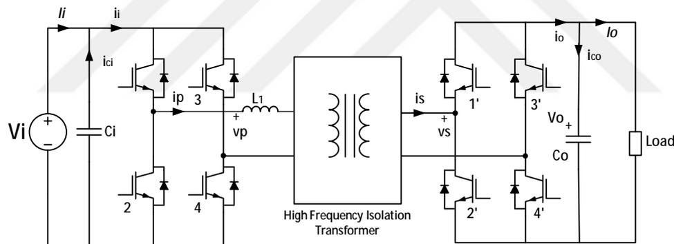
Figure 2.2. SPDAB circuit scheme
