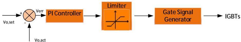
Figure 3.4. The control structure of DAB DC-DC converter
