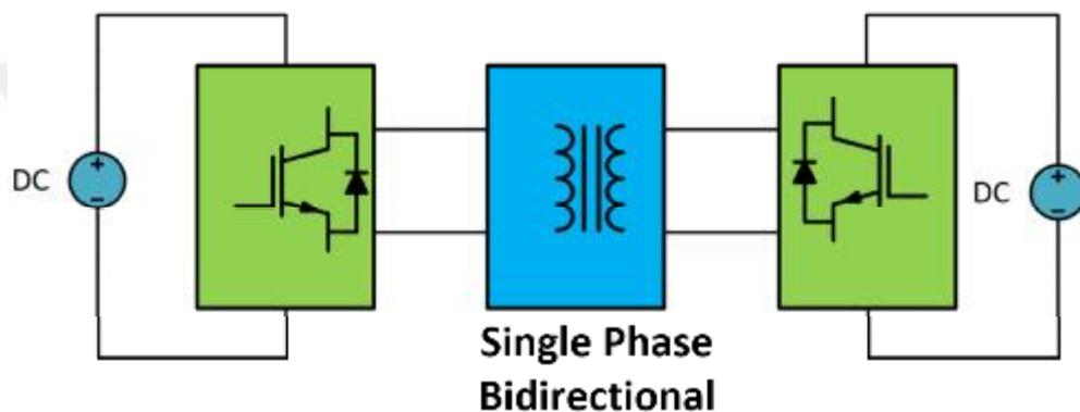
Figure 1.11. Topology B circuit block scheme
