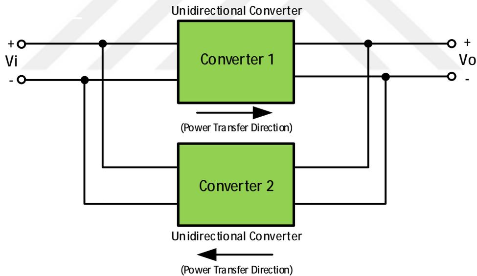
Figure 2.1. The principle construction of bidirectional converter
