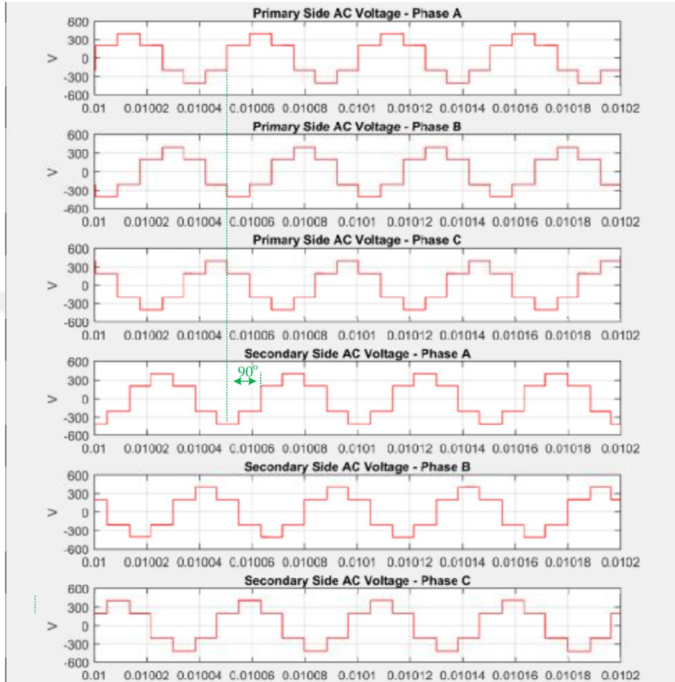
Figure 4.3. The AC voltages of primary and secondary side of the transformer before reaching to set output DC voltage
