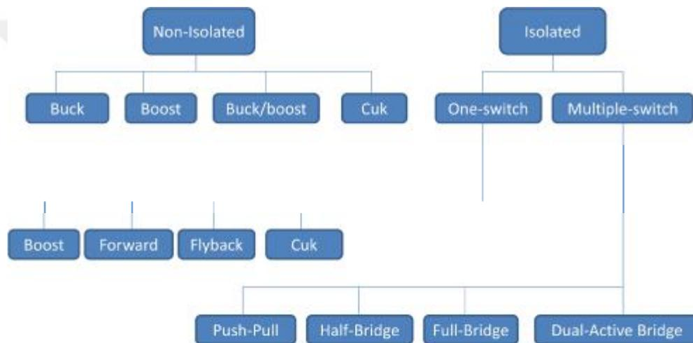
Figure 1.1. General list of common used DC-DC converters
