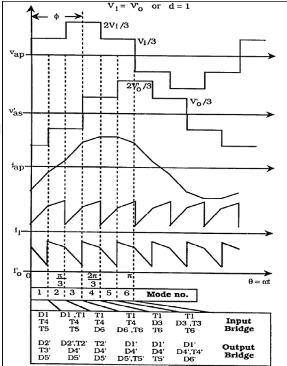
Figure 2.11. The idealized waveforms of phase shift modulation for TPDAB in region II (Kheraluwala et al., 1991)
