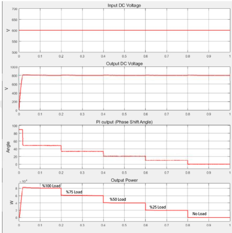
Figure 4.15. The system response to load changes
