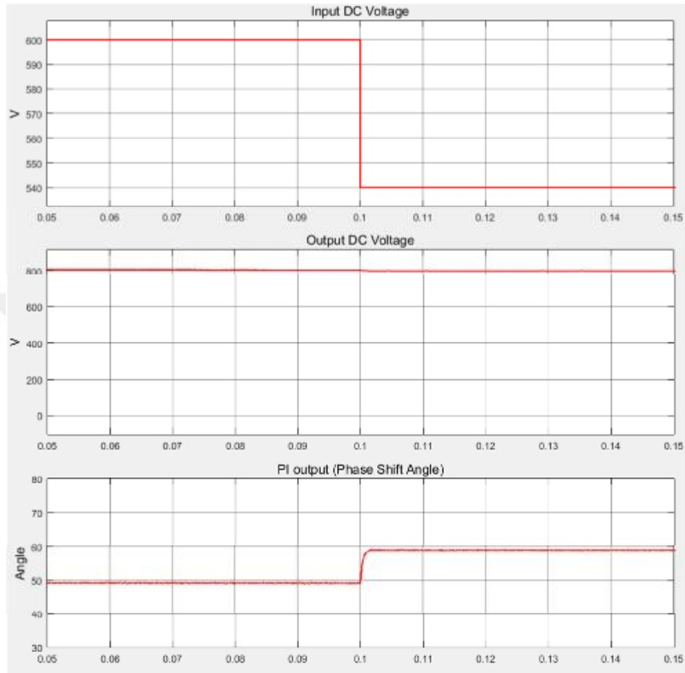
Figure 4.11. The system response to decreasing input DC voltage
