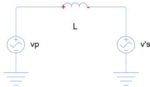
Figure 2.4. The derivative equivalent circuit of SPDAB (Segaran et al., 2008)
