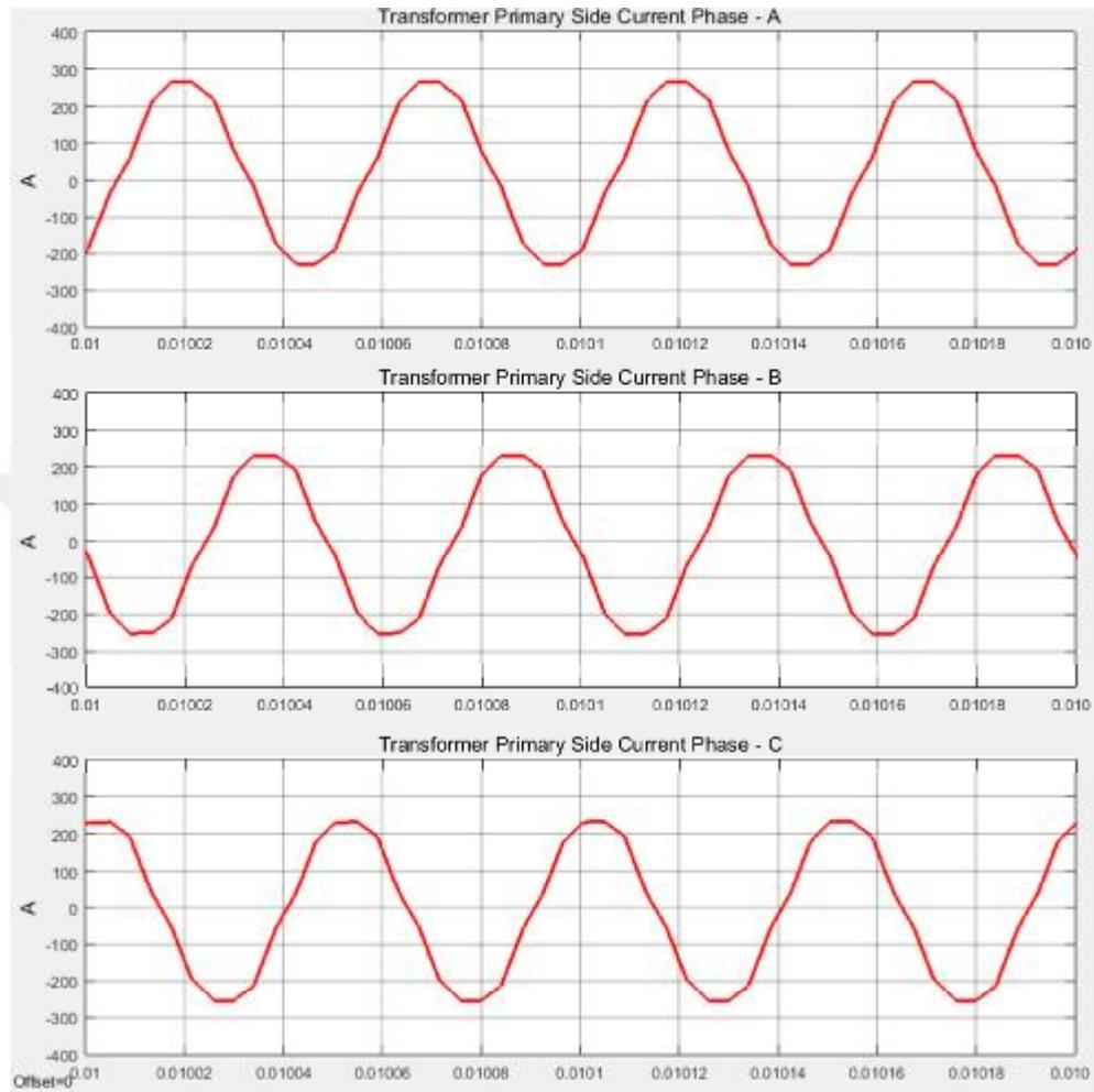
Figure 4.5. The AC currents of primary side of the transformer before reaching to the set output DC voltage
