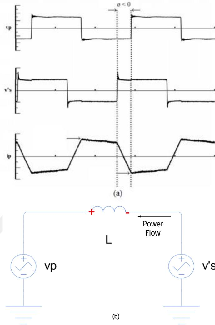
Figure 2.6. Waveforms (a) and power flow direction (b) with applied negative phase shift
