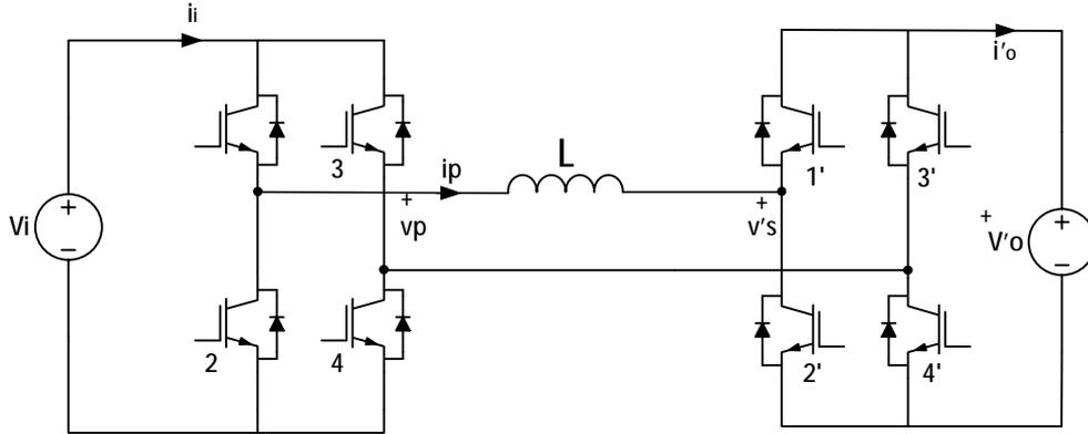
Figure 2.3. Primary referred equivalent circuit of SPDAB
