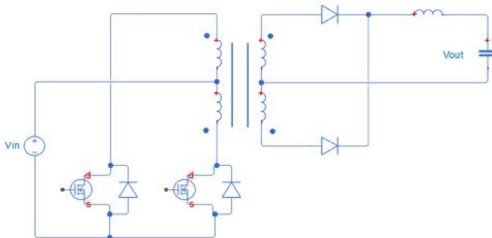
Figure 1.5. Basic push-pull converter circuit
