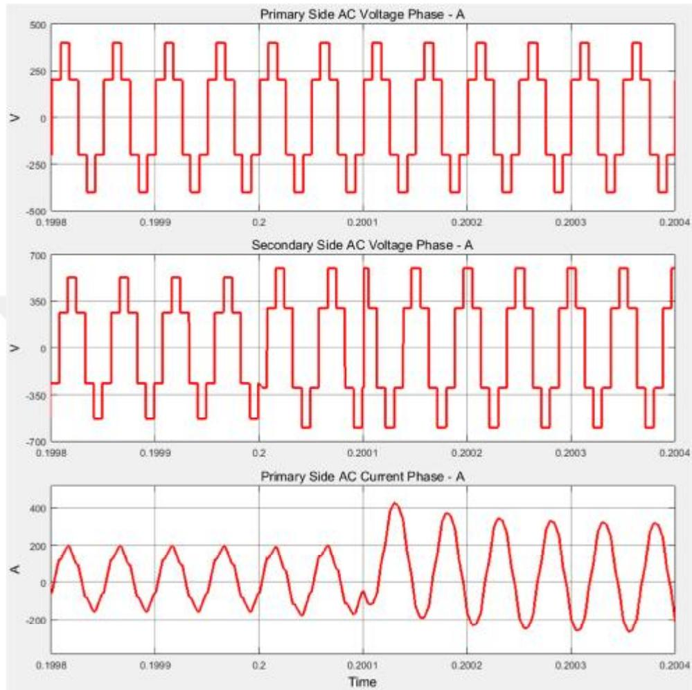
Figure 4.8. The waveforms of increasing output DC voltage
