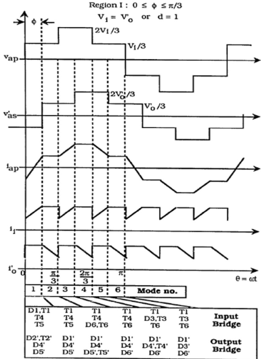
Figure 2.10. The idealized waveforms of phase shift modulation for TPDAB in region I (Kheraluwala et al., 1991)
