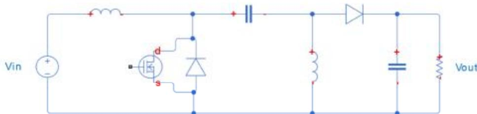
Figure 1.7. Basic SEPIC converter circuit
