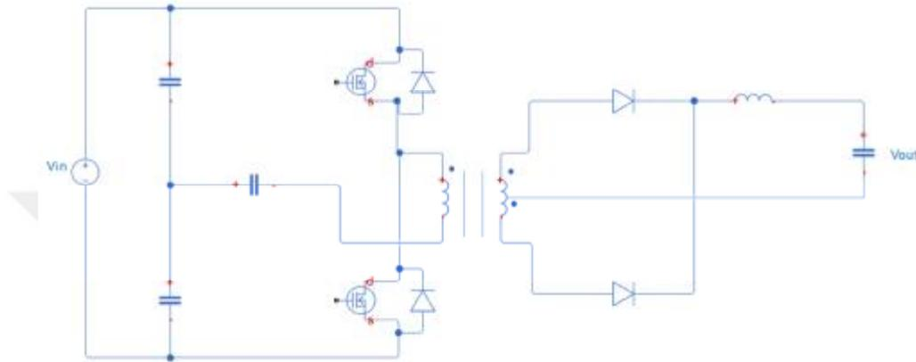
Figure 1.8. Basic half-bridge converter circuit
