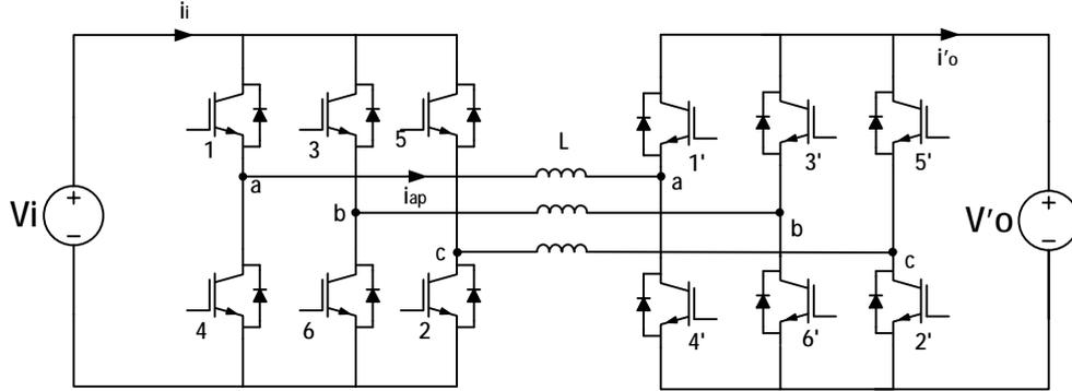
Figure 2.9. The primary referred equivalent circuit diagram of TPDAB converter
