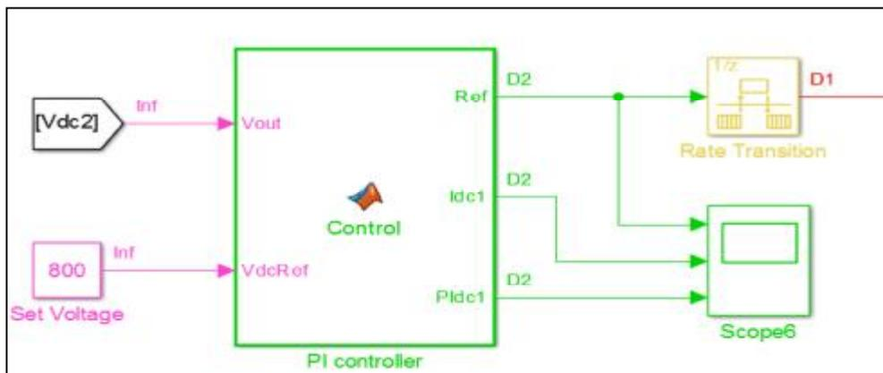
Figure 3.6. The PI controller block in MATLAB/Simulink
