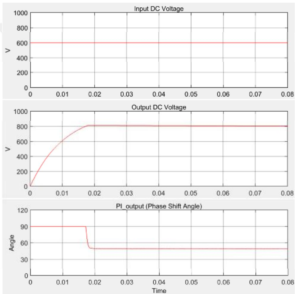
Figure 4.2. The startup input DC voltage, output DC voltage and phase shift angle waveforms
