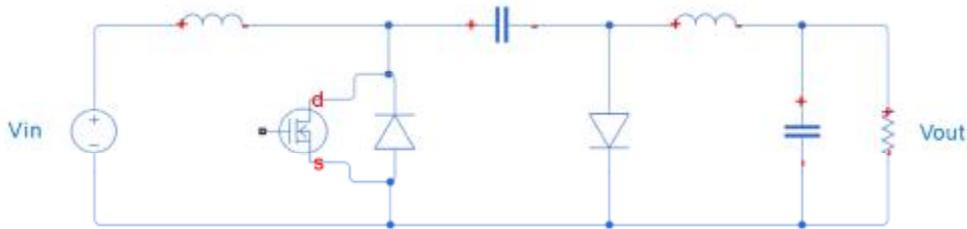
Figure 1.6. Basic CUK converter circuit
