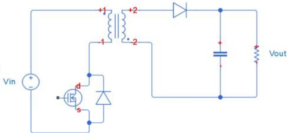
Figure 1.3. Basic flyback converter circuit
