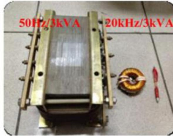
Figure 3.1. The comparative photos of the 50 Hz and the 20 kHz transformers (Zhao et al., 2014)
