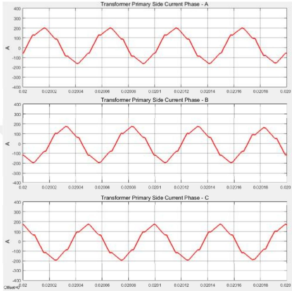
Figure 4.6. The AC currents of primary side of the transformer after reaching to the set output DC voltage
