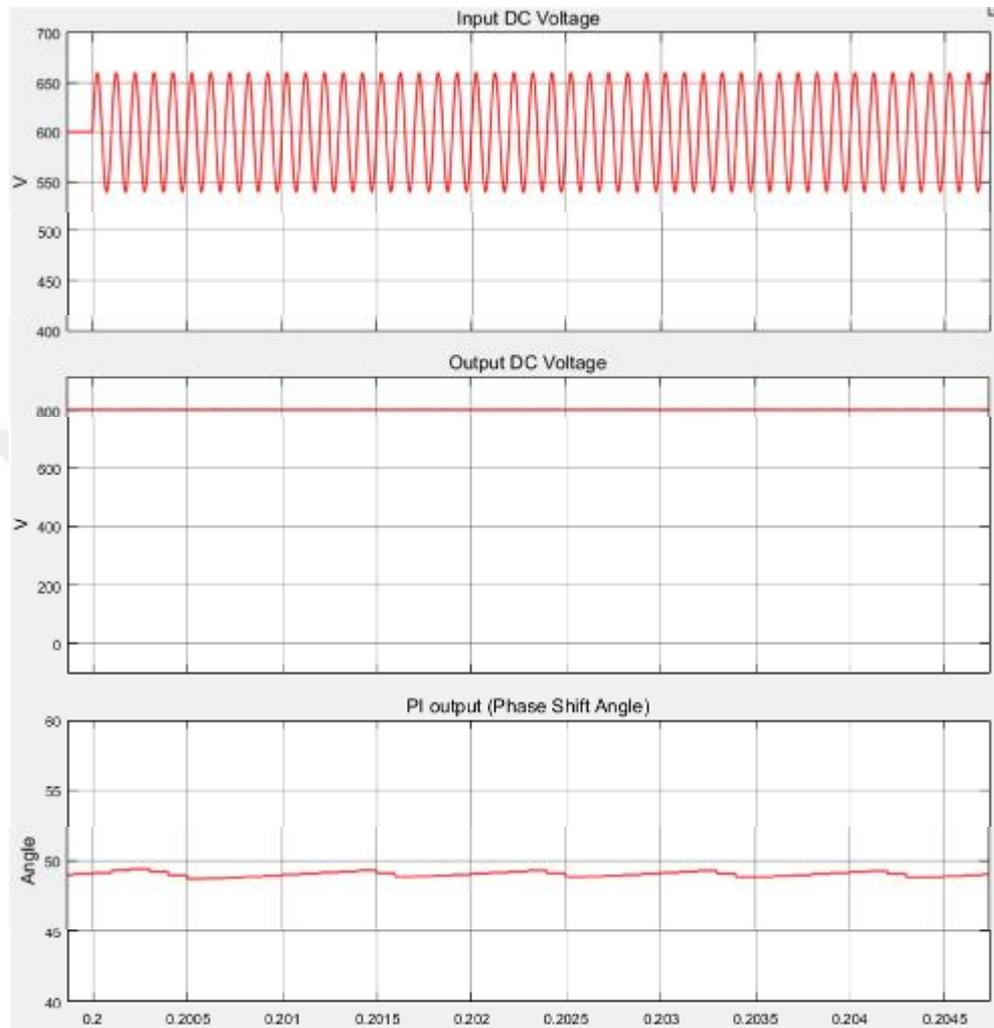
Figure 4.13. The system response to oscillating input DC voltage
