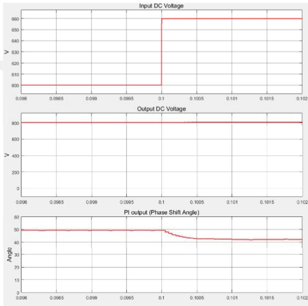
Figure 4.9. The system response to increasing input DC voltage
