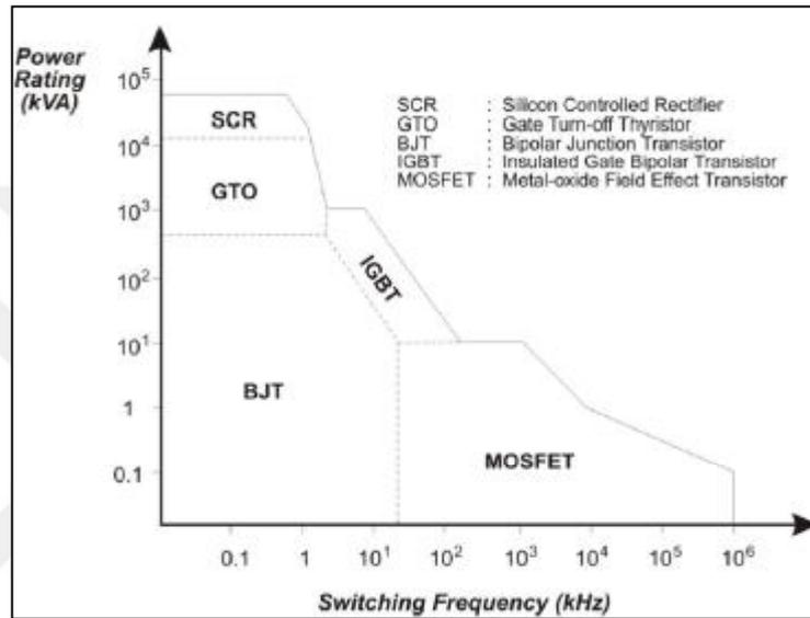
Figure 3.2. Performance limits of gate controlled devices (Barnes, 2003)
