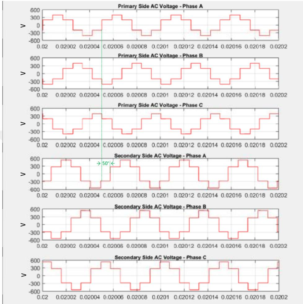
Figure 4.4. The AC voltages of primary and secondary side of the transformer after reaching to set output DC voltage
