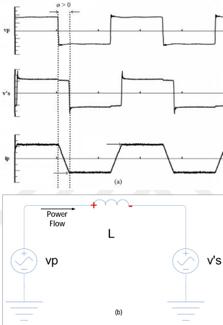
Figure 2.5. Waveforms (a) and power flow direction (b) with applied positive phase shift
