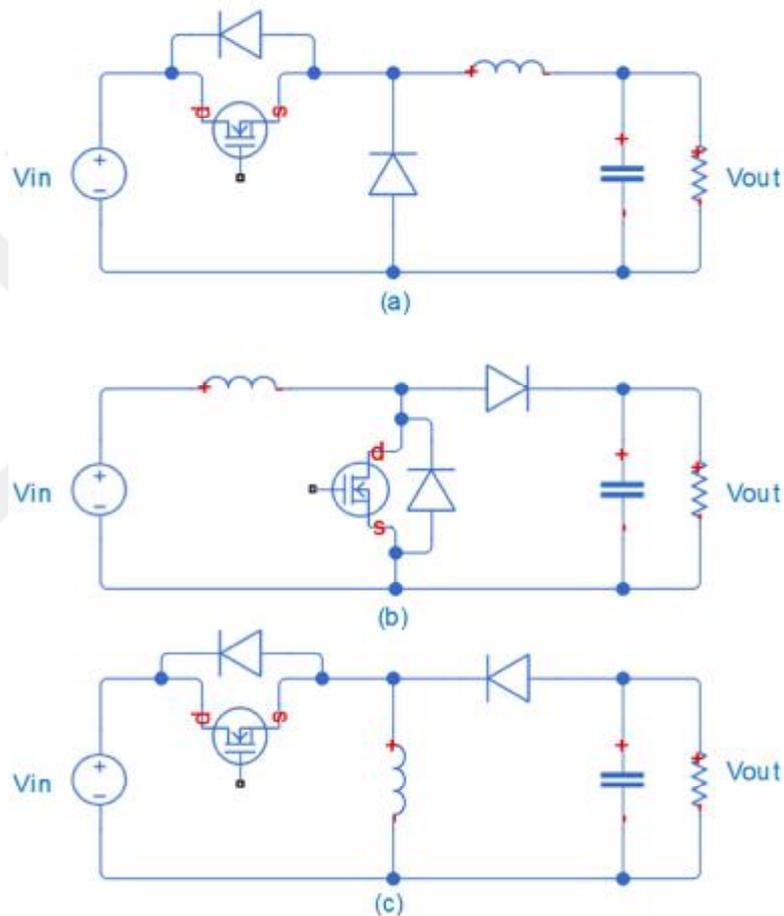
Figure 1.2. Buck (a), boost (b), buck-boost converter circuits
