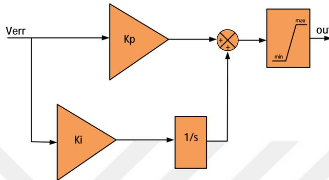
Figure 3.5. PI controller block diagram
