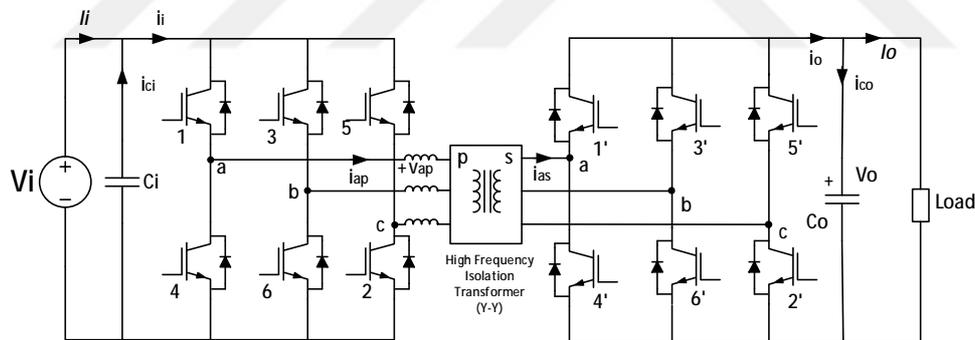
Figure 2.8. The basic circuit scheme of TPDAB converter
