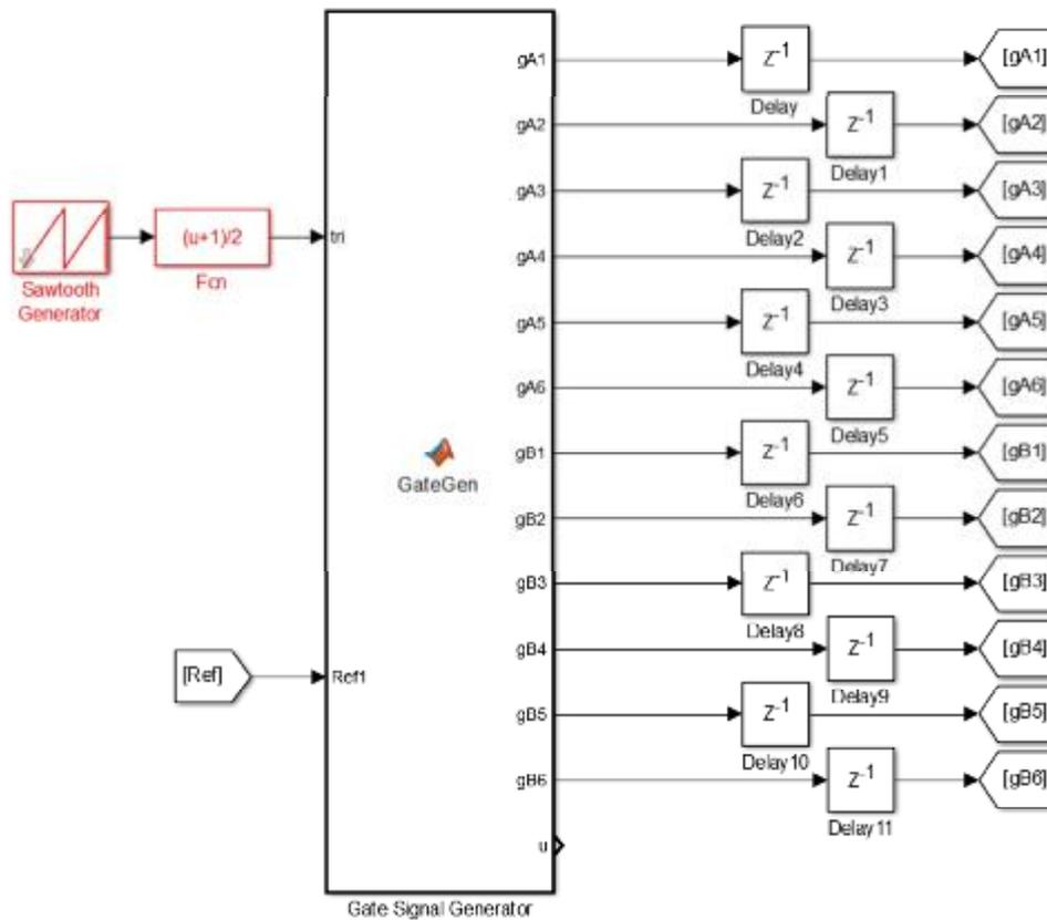
Figure 3.9. Gate signal generator block in Simulink
