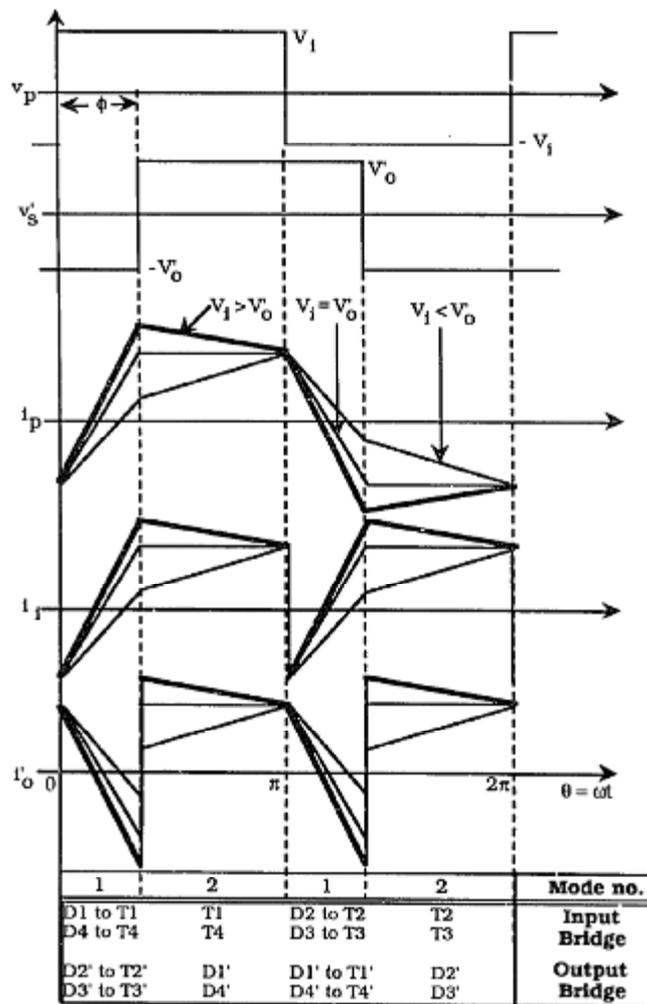
Figure 2.7. Idealized waveforms of phase shift modulation for SPDAB (Kheraluwala et al., 1991)
