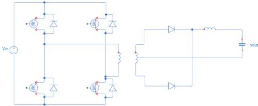
Figure 1.9. Basic full-bridge converter circuit
