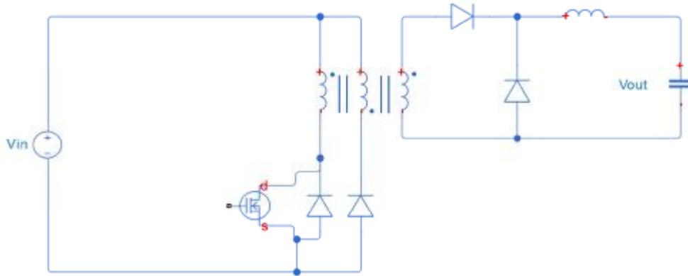
Figure 1.4. Basic forward converter circuit
