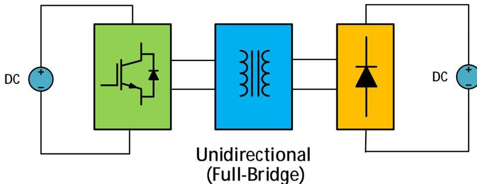
Figure 1.10. Topology A circuit block scheme
