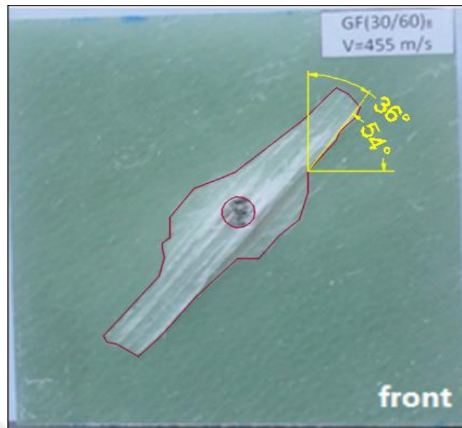
c) stacking sequence of [30^\circ/60^\circ]_{A8} , V_1 = 455 m/s
