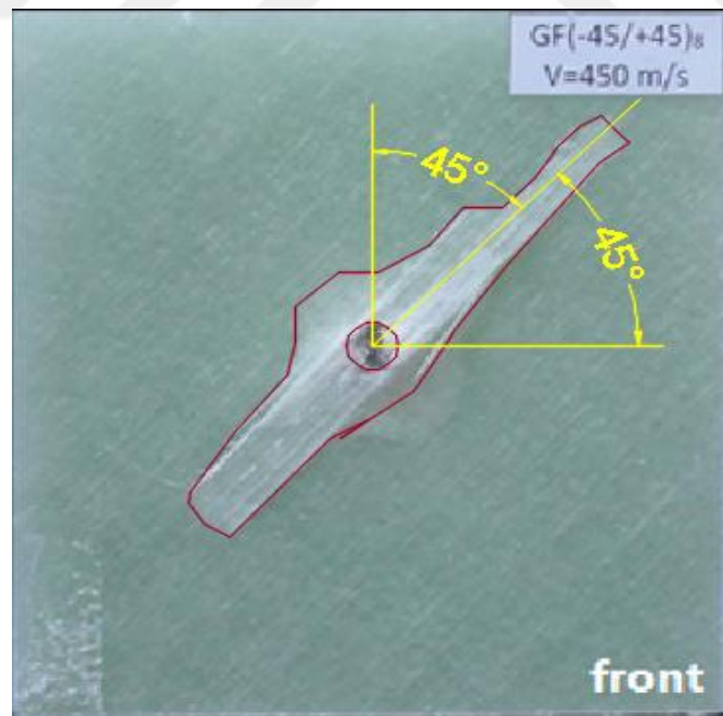
b) stacking sequence of [-45^\circ/+45^\circ]_{A8} , V_1 = 450 m/s
