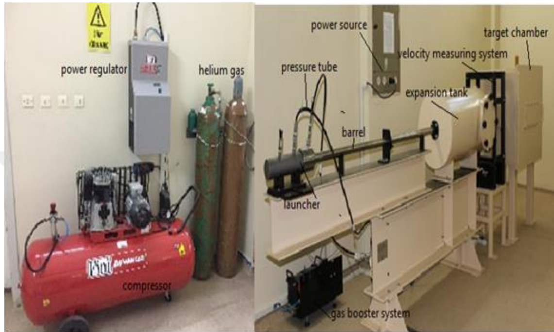
Figure 2.24. Ballistic testing system (Single- stage gas -gun).
