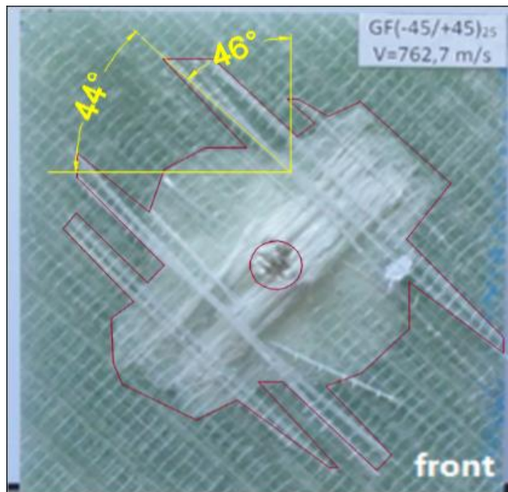
b) stacking sequence of [-45^\circ/+45^\circ]_{A25} , V_2 = 762.7 m/s
