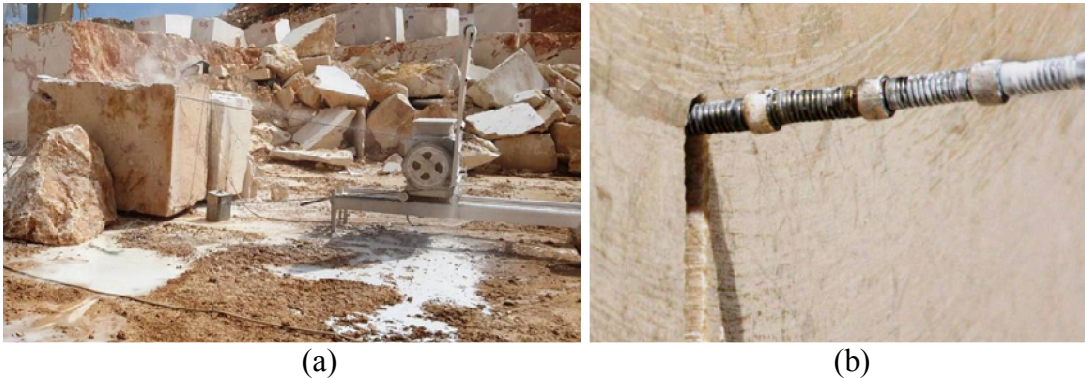
Figure 3.11 : (a) The visuals from the fields and (b) Diamond wire cutting method.
