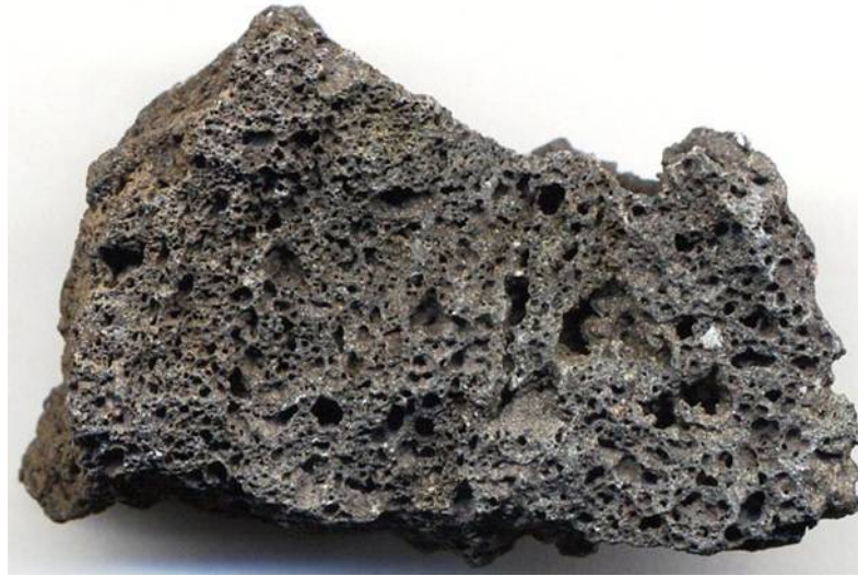
Figure 4.8 : The image of the vesicular structure of the Ankara andesite rock.
