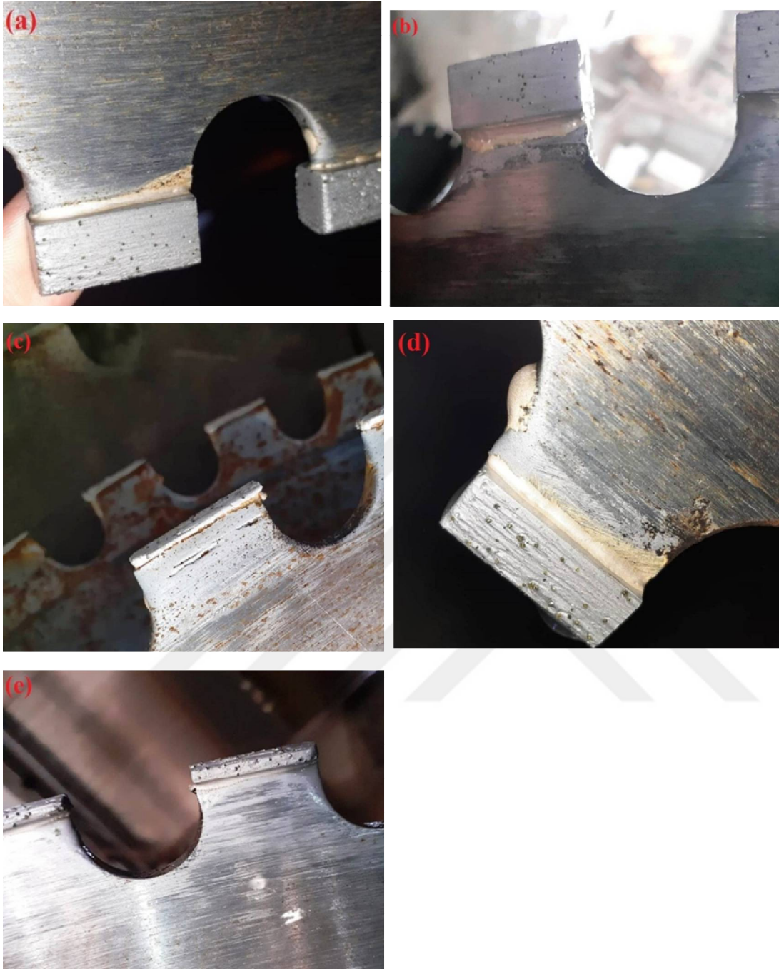
Figure 4.12 : The images of segment until cutting process a) C -70 m2 b) CAA -70 m2 c) C-820 m2 d) CAA-820 m2 e) CAA-1400 m2.
