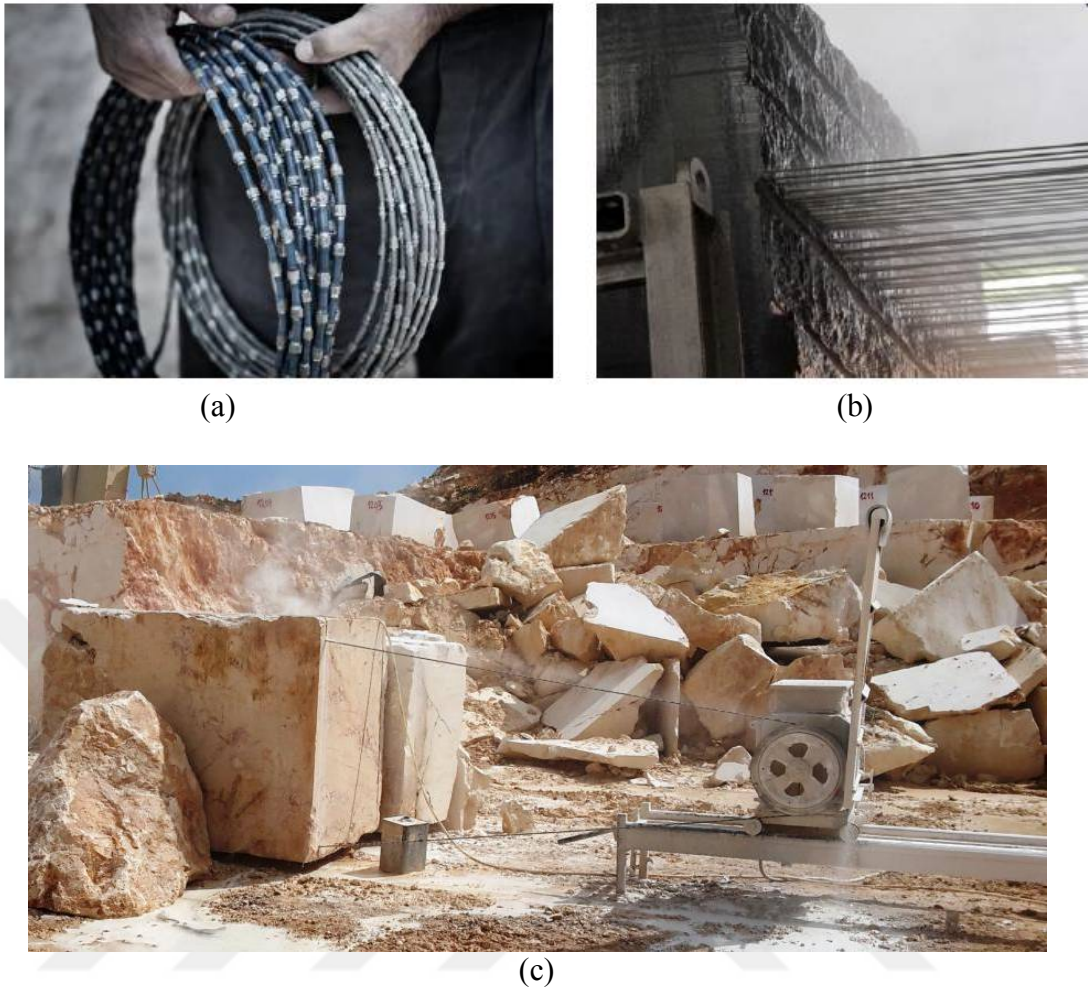
Figure 1.7 : The diamond wire machines a) diamond wire b) multiwire c) monowire.
