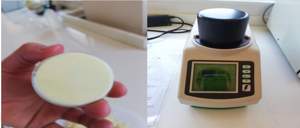
Figure 3.9 Kashar samples cheese was put into special glasses in left and hunter lab color measurement device in right.
