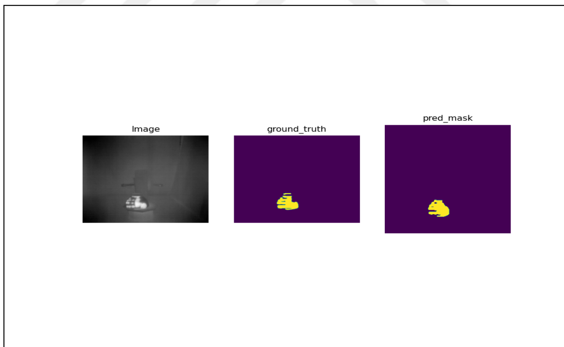
Figure 4.15: The result of semantic segmentation for the object “bowl” by U-net.
