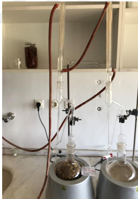
Figure 2.3: Clevenger apparatus for hydrodistillation.
