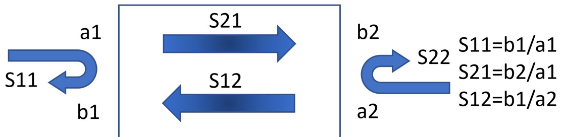
Figure 3.1 Representation of S parameters in a 2-port system
