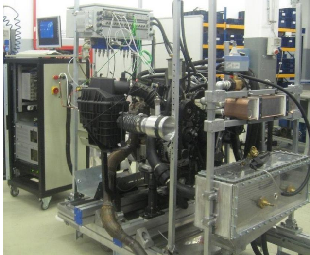
Figure 2.1 : Test engine before connecting to the dynamometer.
