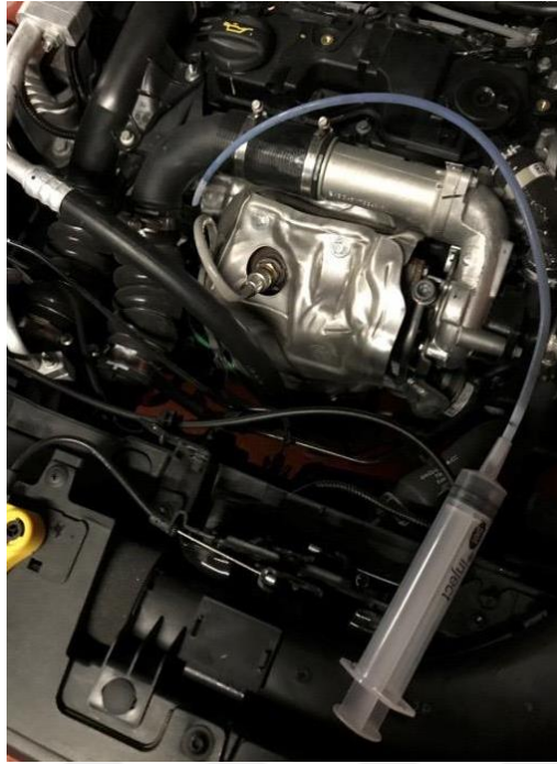
Figure 2.4 : Sampling from oil level indicator housing.
