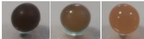
Figure 3.4: Fe-BTC/Alginates changing back to original color during release process.
