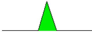
Fig. 1.4: Less concentration of injected compound can be interpreted by less area under the chromatogram (63)
