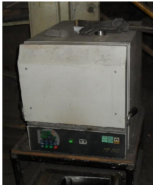
Figure 4.14 Electrical Box Type Furnace
