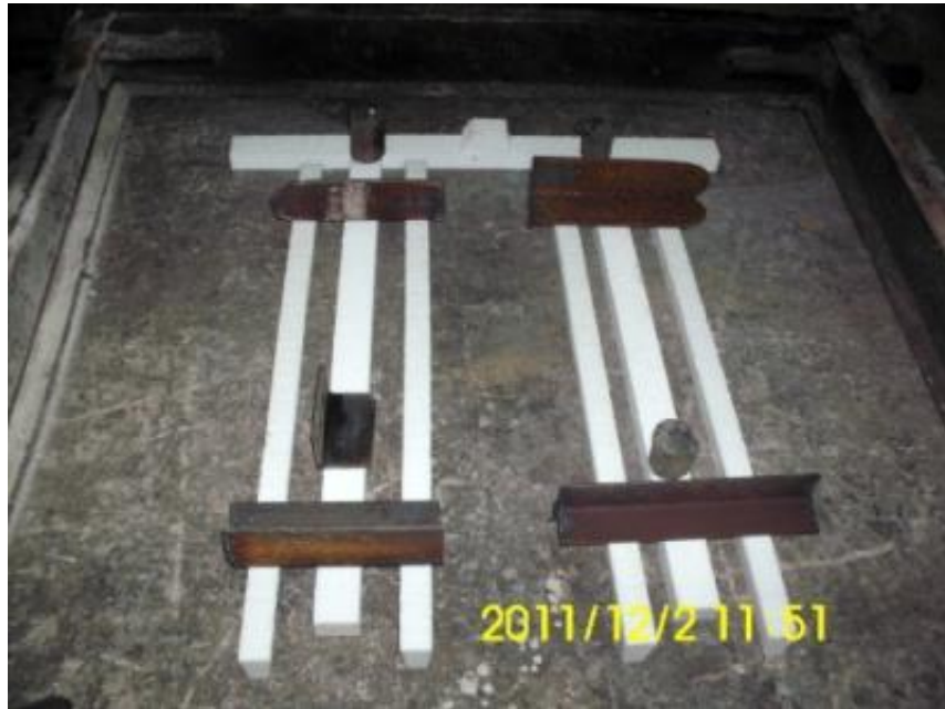
Figure 4.1 The Pattern of the Gating System in Lowest Flask
