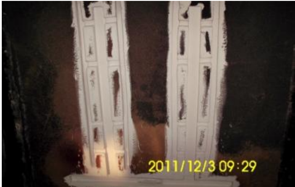
Figure 4.7 Painted Cavity of Gating System (Lowest Flask)
