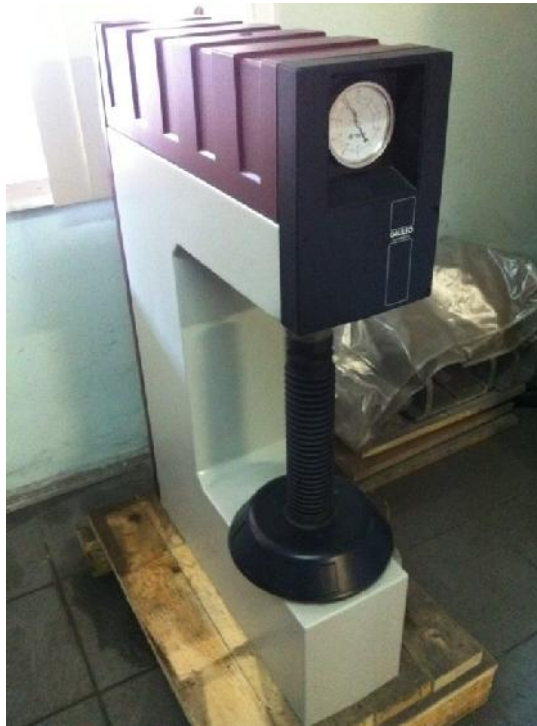
Figure 7.1 Rockwell Hardness Tester
