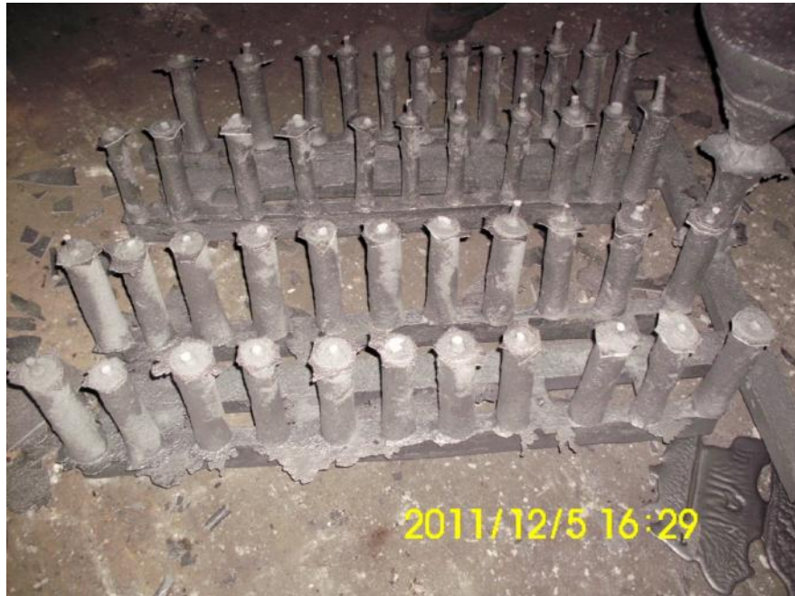
Figure 4.12 Specimens after shakeout
