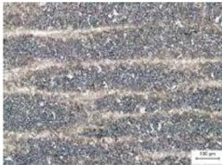
Figure 2.4 The block segregation on a hot work tool steel. [17]
