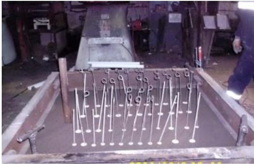
Figure 4.5 Formation of the Gas Release Holes
