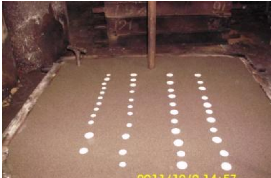
Figure 4.4 Molding of Cope (First Stage)
