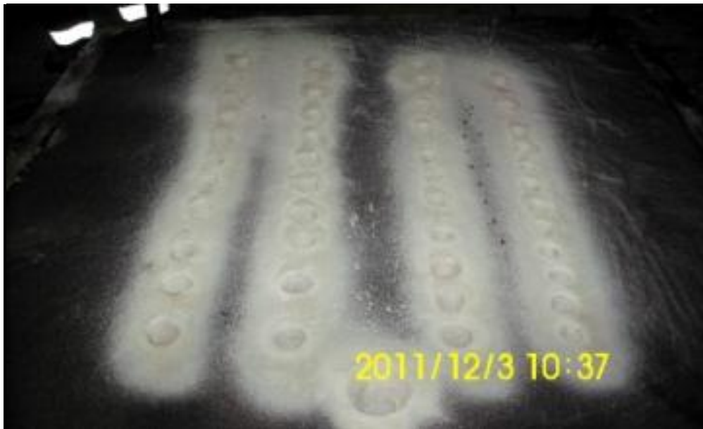
Figure 4.8 The view of the Cope after Painting
