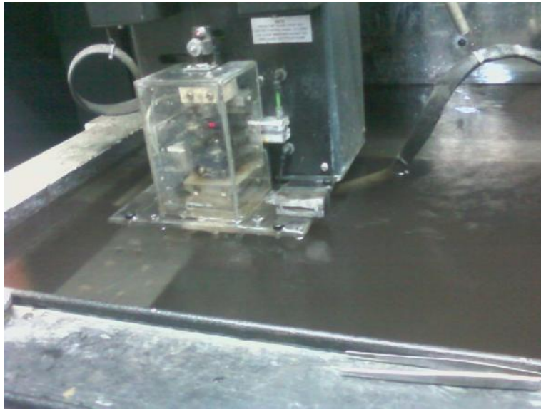
Figure 7.4 V- Notch Machining by Electrical Discharge Machining
