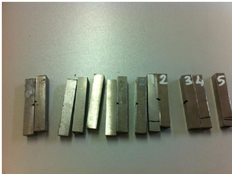
Figure 7.5 Charpy V- Notch Specimen
