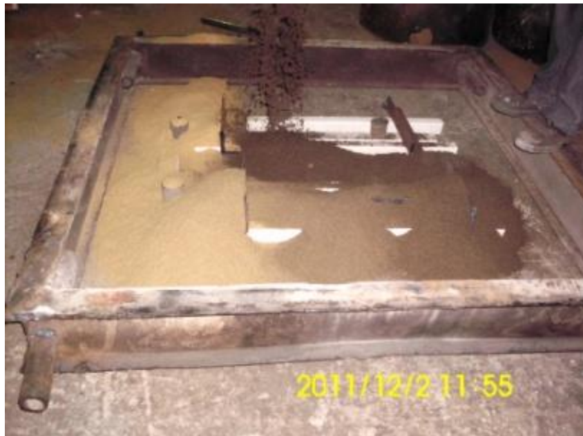
Figure 4.2 The Filling of the Drag with Sand
