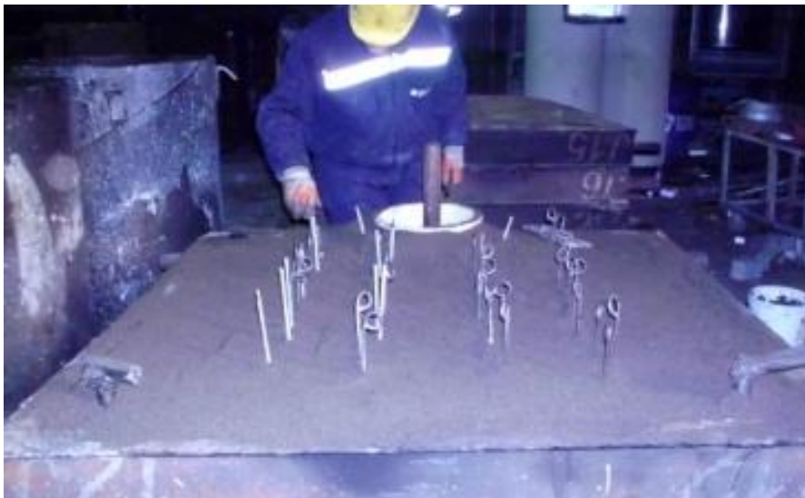
Figure 4.6 Molding of Cope
