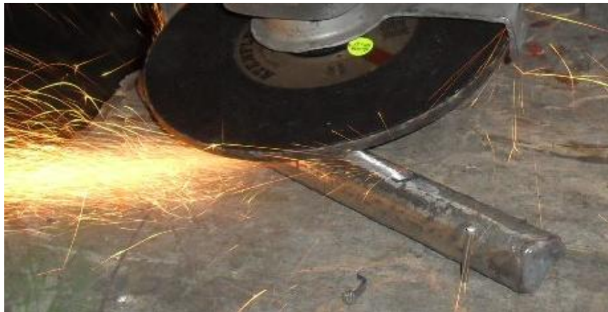
Figure 4.13 The Surface Cleaning of the Billets by Grinding
