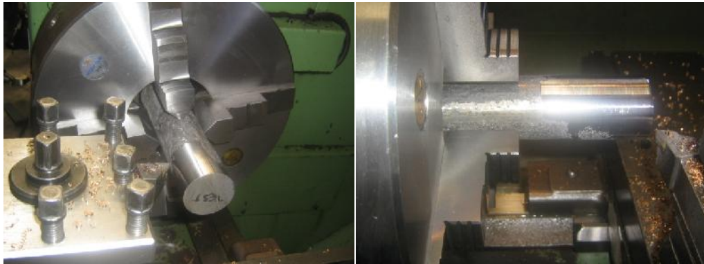
Figure 6.1 Turning Operation of the Specimens
