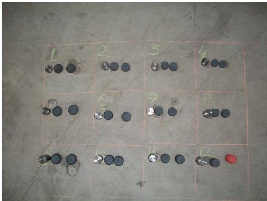
Figure 6.7 Grouped Billets After Forging
