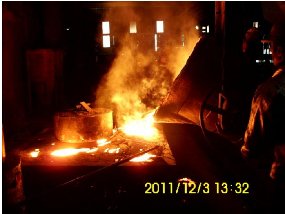
Figure 4.11 Pouring of tool steel into the mold
