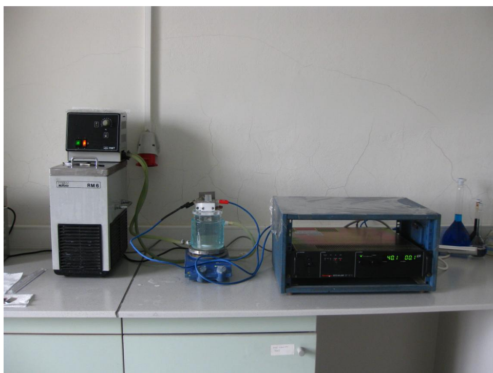
Figure 3.2: Anodization setup used for oxalic acid anodizing
