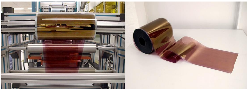
Figure 1.3 Example of a roll-to-roll coated OPV device on a PET foil (Polyethylene Terephthalate) substrate.[7]
